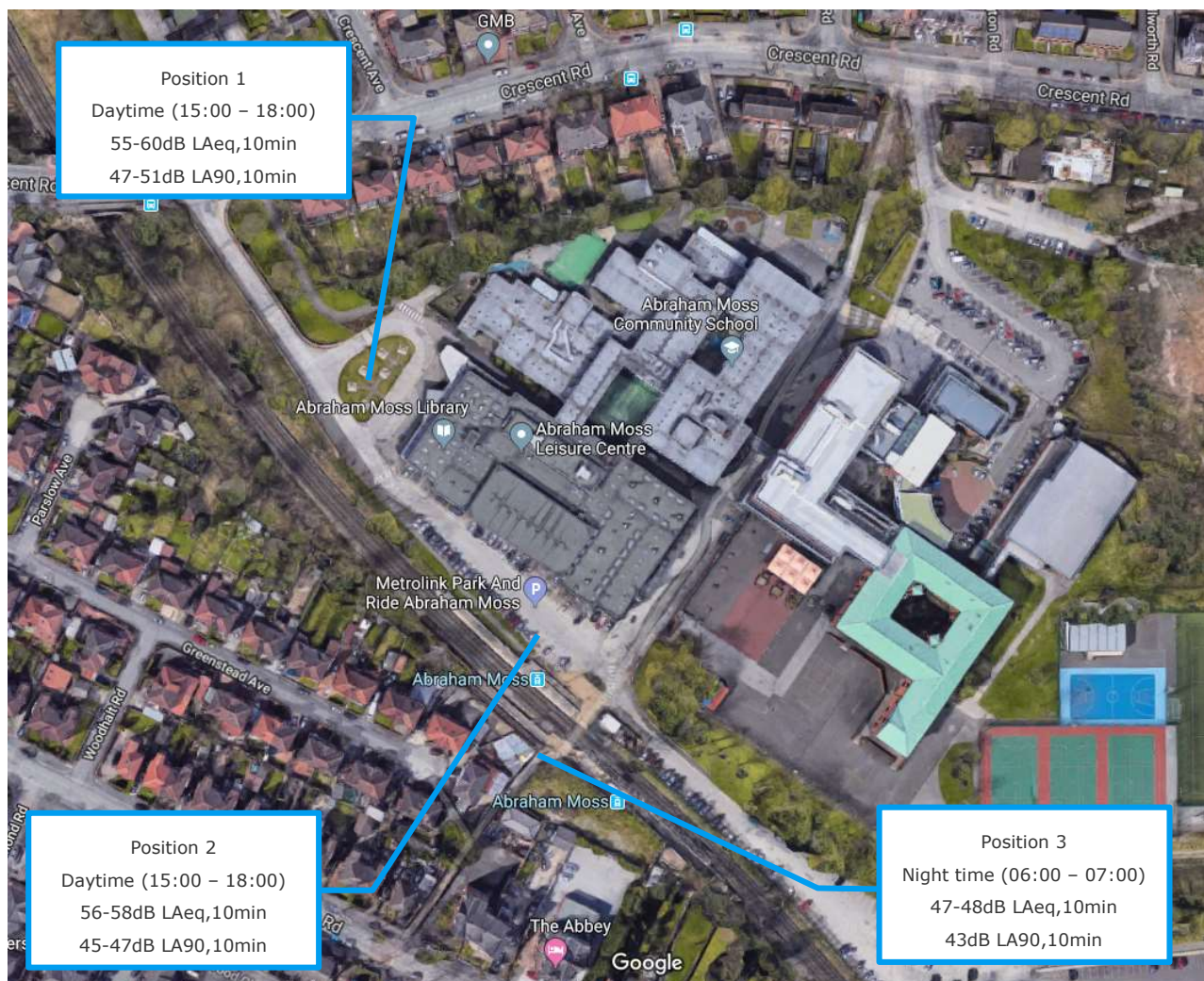
Figure 1 – Survey positions and measured levels
