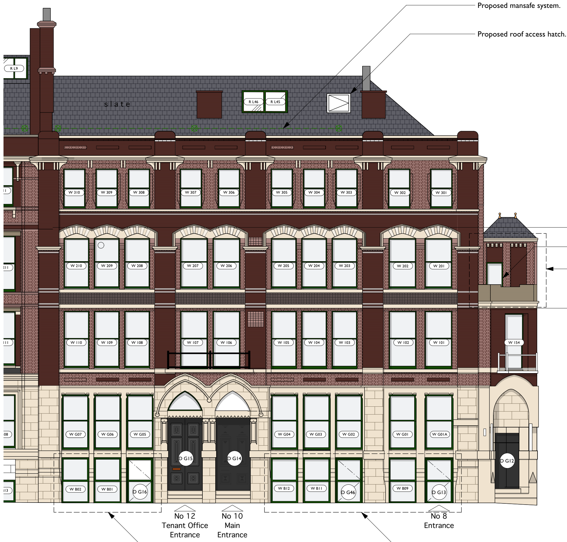
Proposed Elevation 2 - Newton Street Scale 1:150
