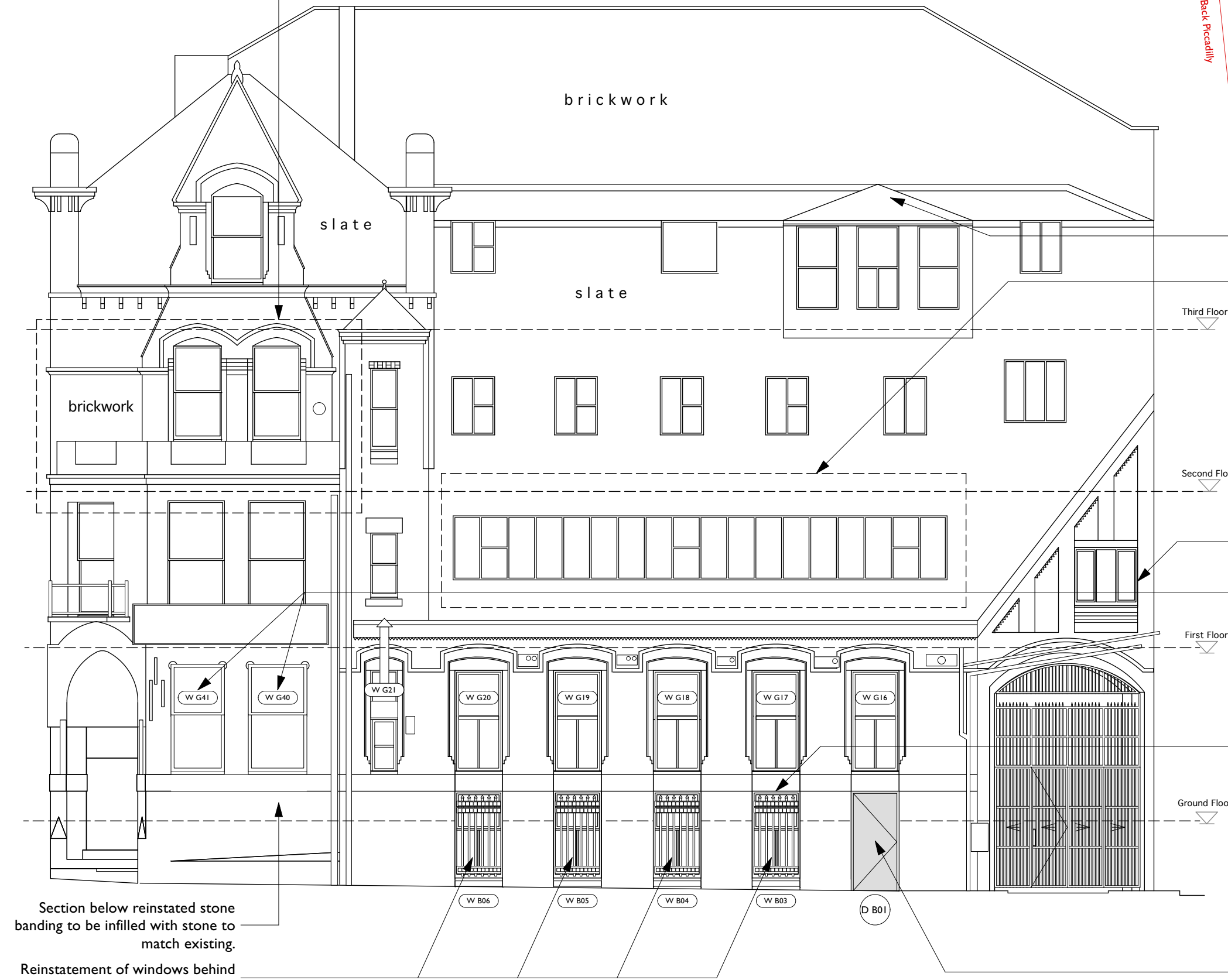
Proposed Elevation - Back Piccadilly Scale 1:100
