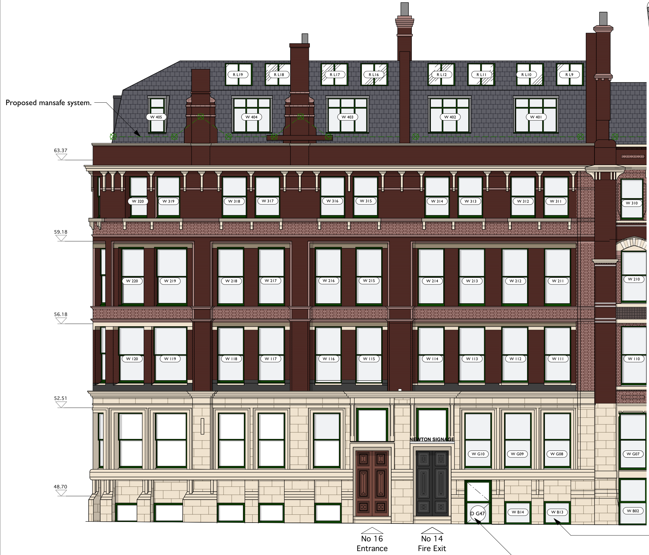
Proposed Elevation I - Newton Street Scale 1:150
