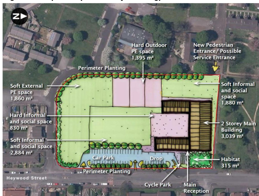
Figure 2.2: Option 1 (Two Storey Building)
