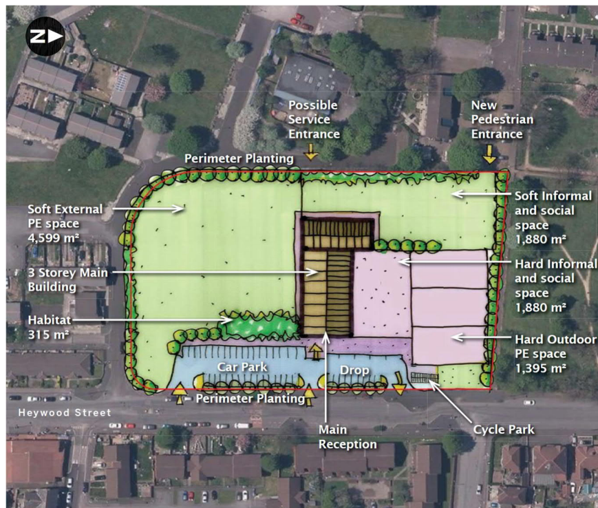
Figure 2.3: Option 2 (Three Storey Building)
