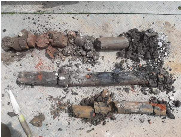
Photograph 1: Cores recovered from BH1.
