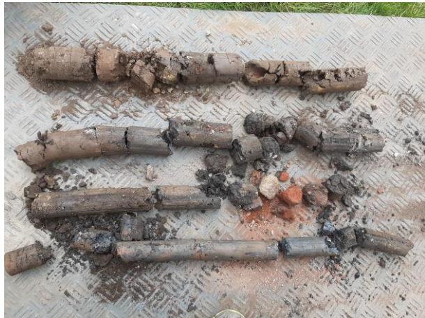
Photograph 2: Cores recovered from BH2.
