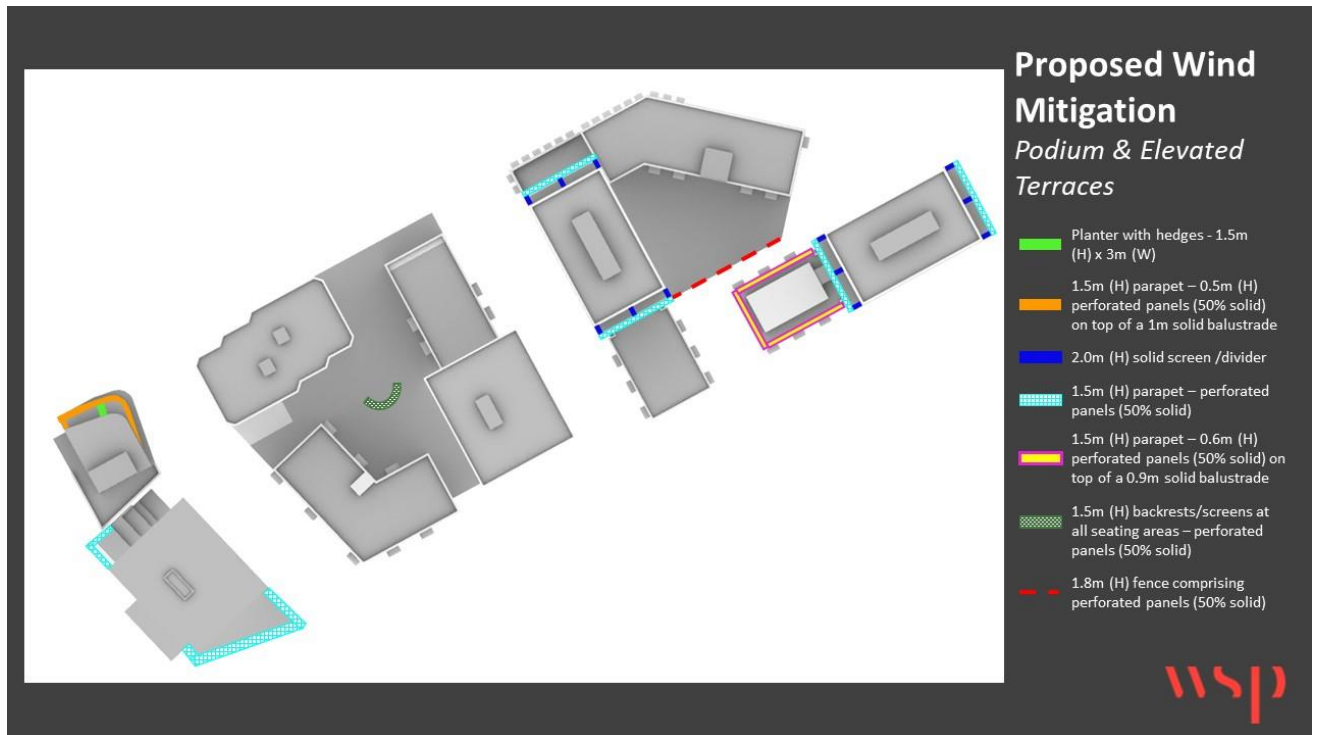
Figure 3-38 – Proposed wind mitigation (podium and elevated terraces).
