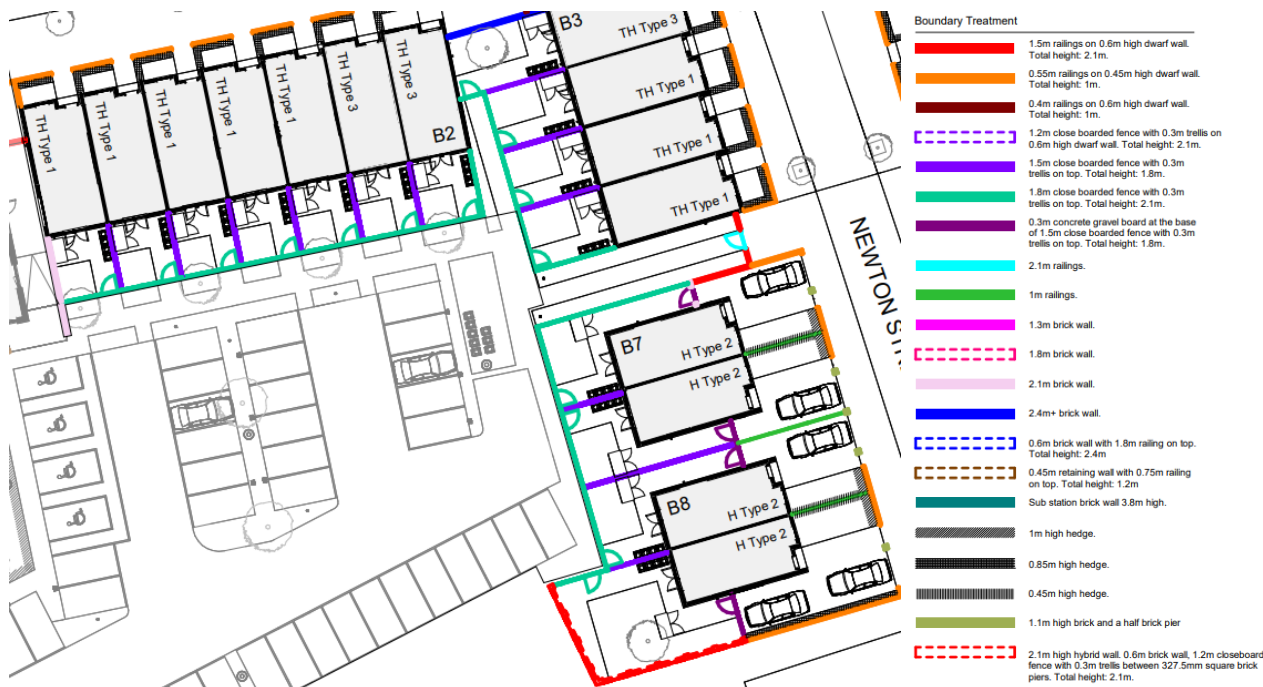
Extract from Proposed Boundary Treatment Plan T8130D0040I3
