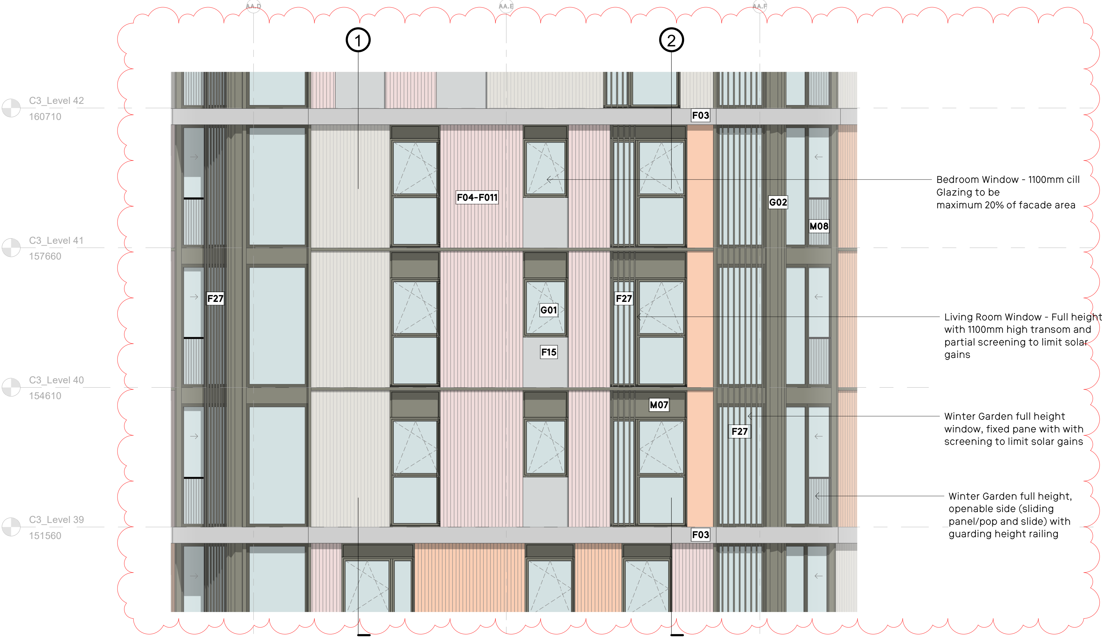
Bay Study, West Elevation Typica; 1: 50
