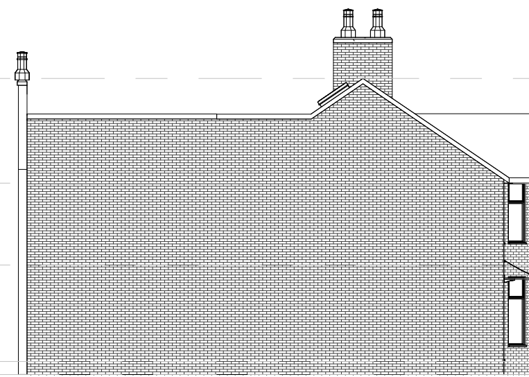
Existing Left-Side Elevation 1 : 150
