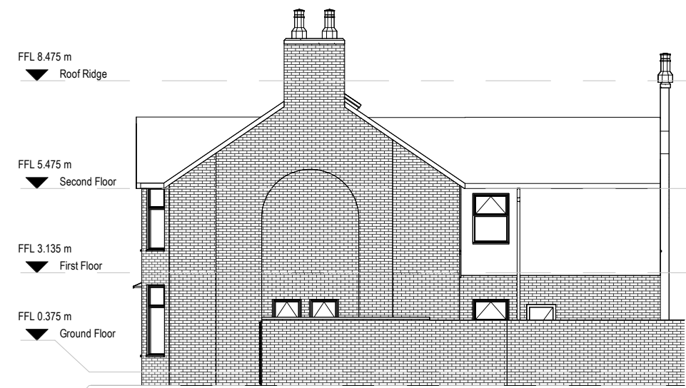
Existing Right-Side Elevation 1 : 150
