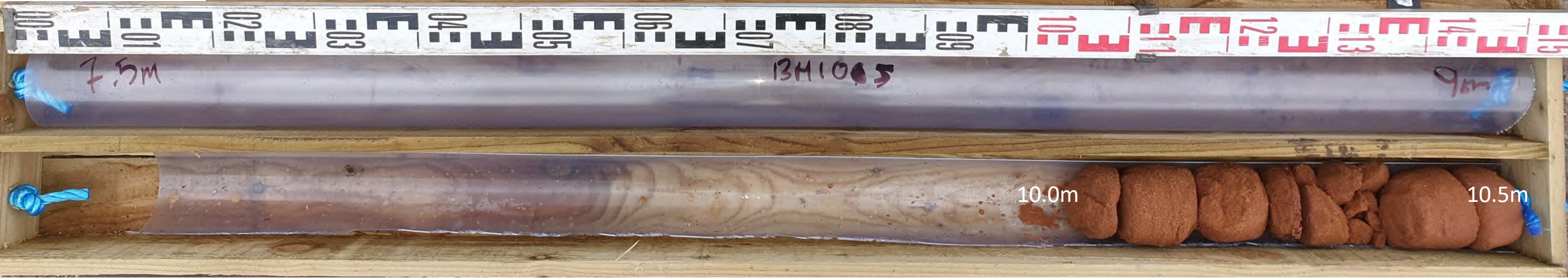
BH105 Box 1 CORE RUN 1 AND 2 7.5m – 10.5m
