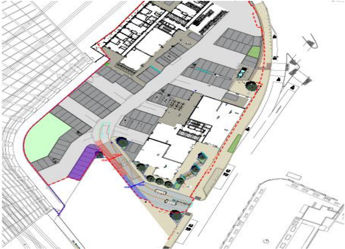
Fig. 2 – Tracked Fire Tender Route into Residential Scheme
