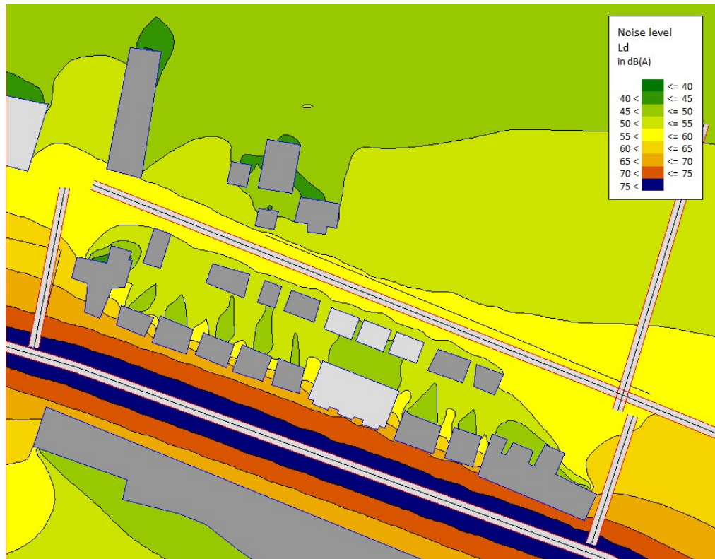
Figure 7 : Night-time Ambient Noise Map (1.5m above ground) -Site and Surroundings
