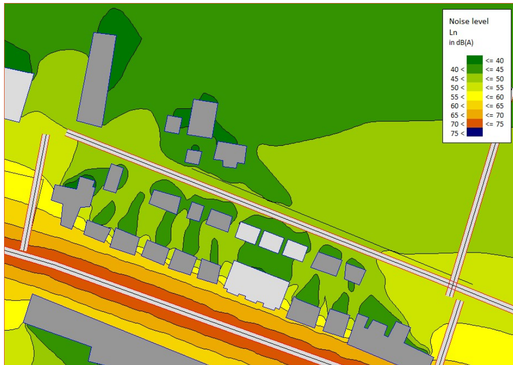
Figure 7 : Night-time Ambient Noise Map (1.5m above ground) -Site and Surroundings
