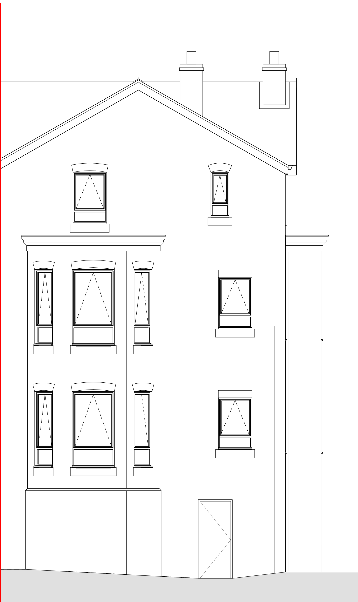
Rear Elevation (Existing) 1 : 50
