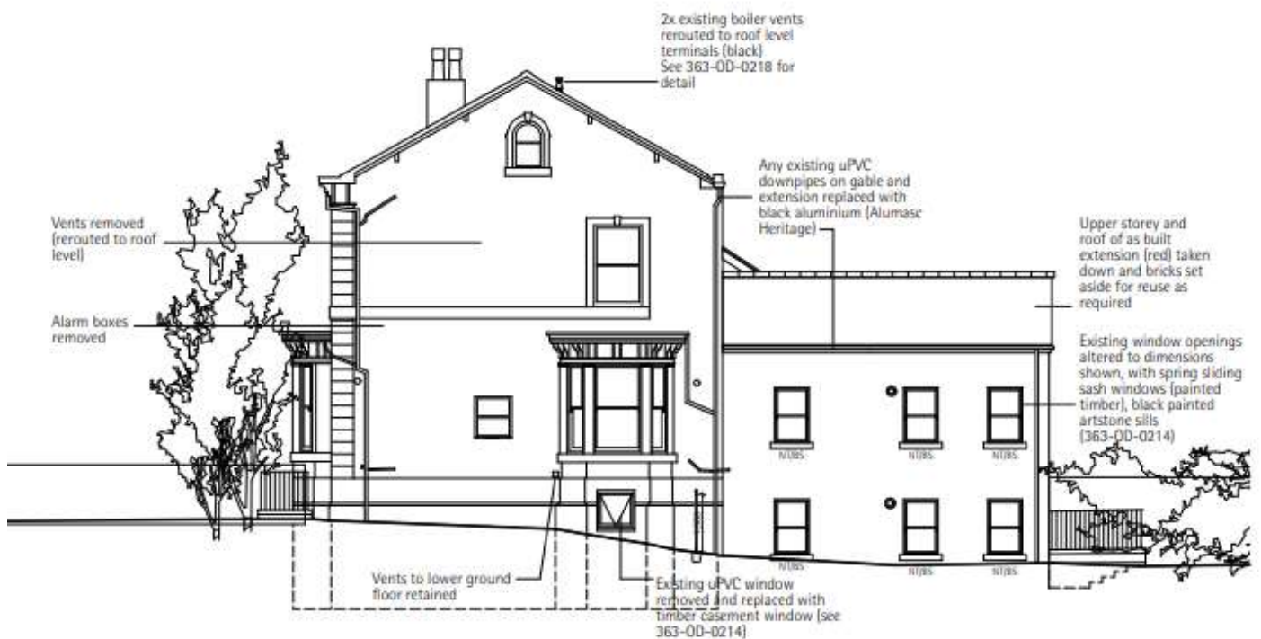
Fig 18. The proposed removal of arched heads which weakens the elevational design.
