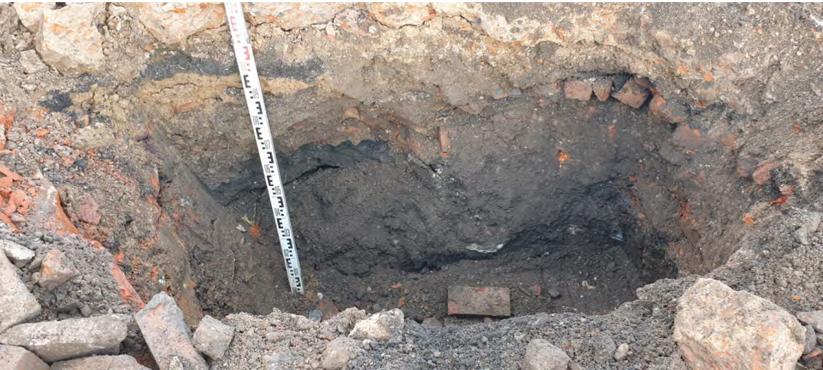
Soil sample obtained for leachate analysis in pit at depth of 1.25m
