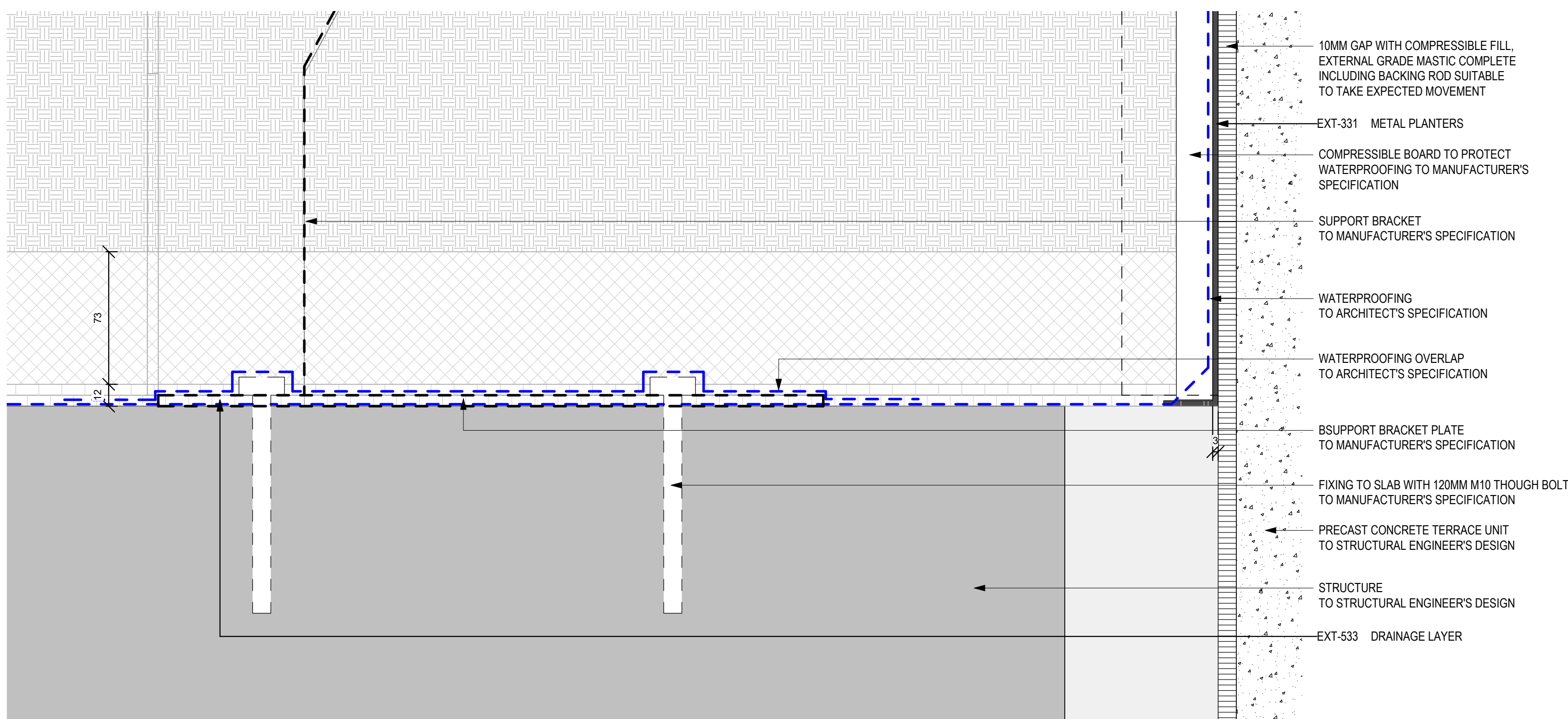
5 TYPICAL METAL PLANTER FIXING DETAIL 1:2
