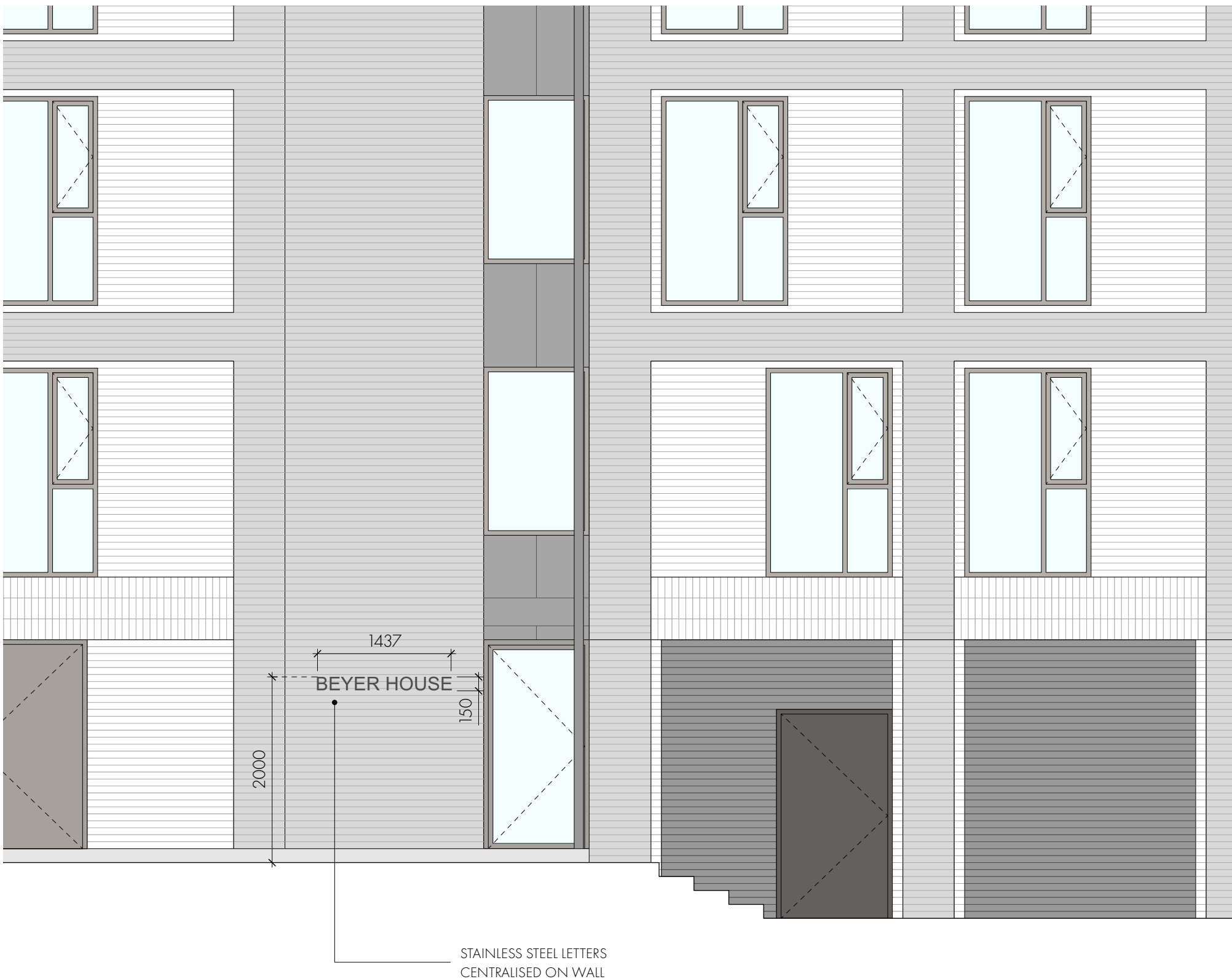
SIGNAGE LOCATION 1 ELEVATION AT 1:50 "BEYER HOUSE"
