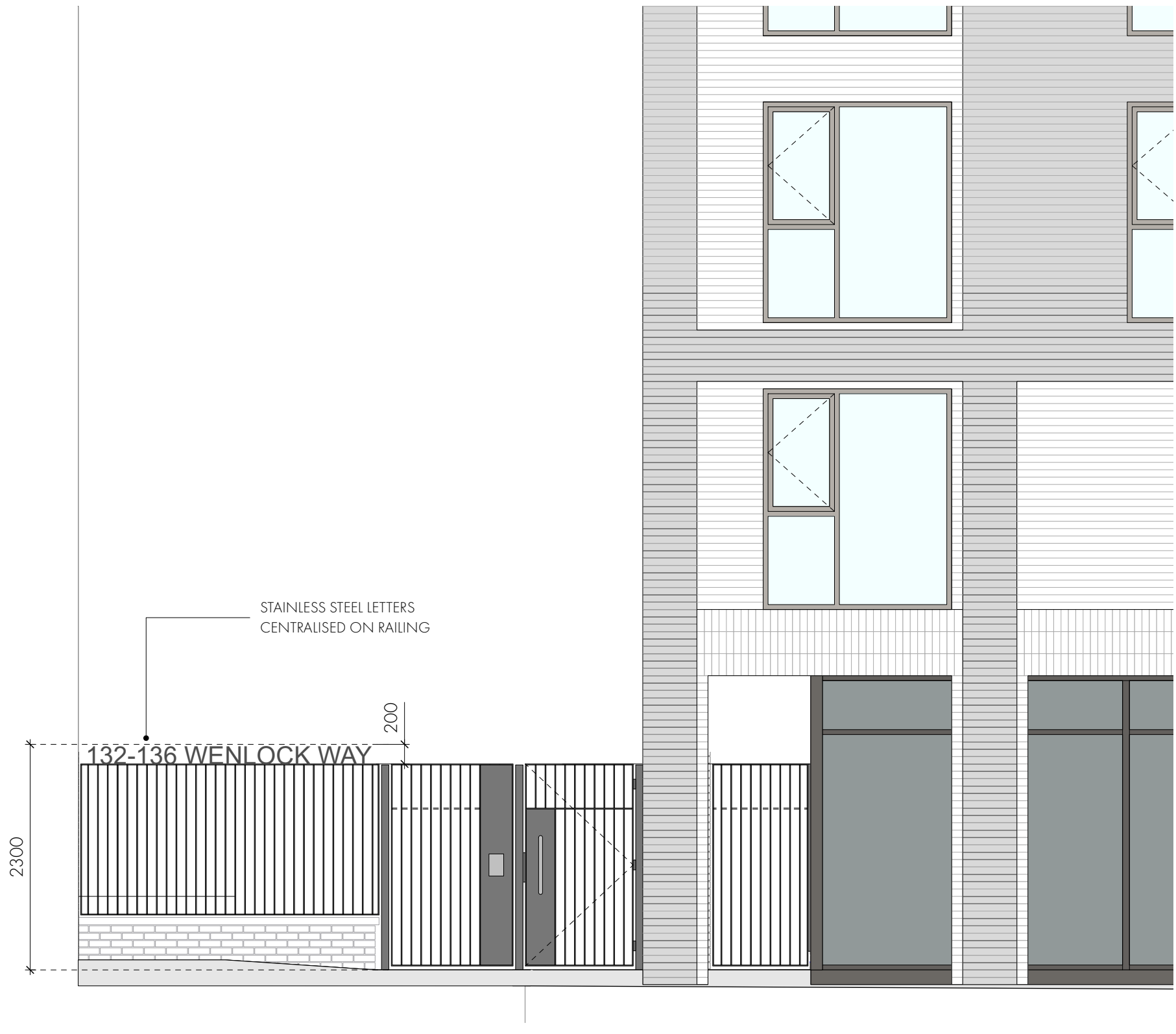
SIGNAGE LOCATION 2 ELEVATION AT 1:50 "132-136 WENLOCK WAY"
