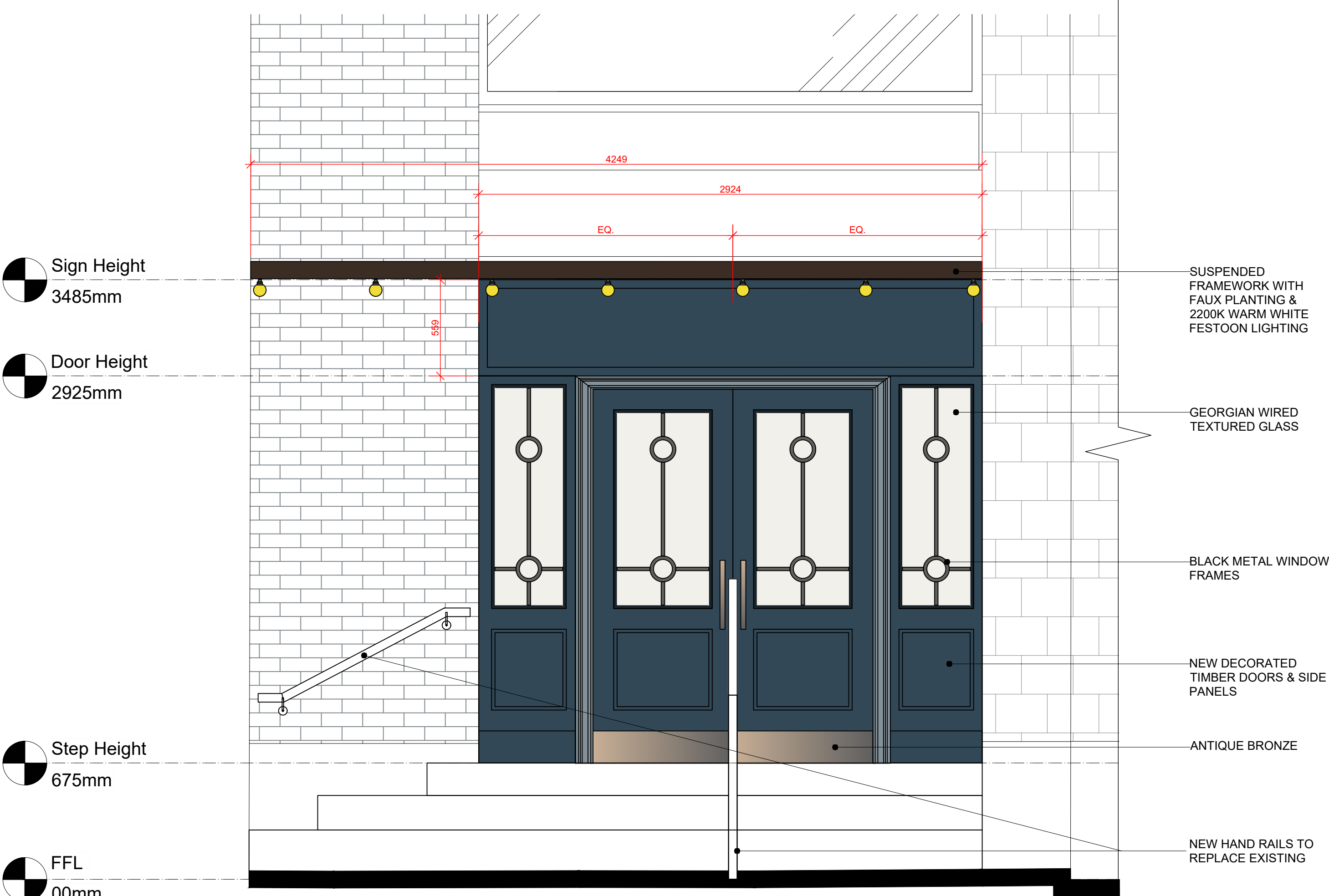
Proposed Front Entrance Detail Scale 1:20
