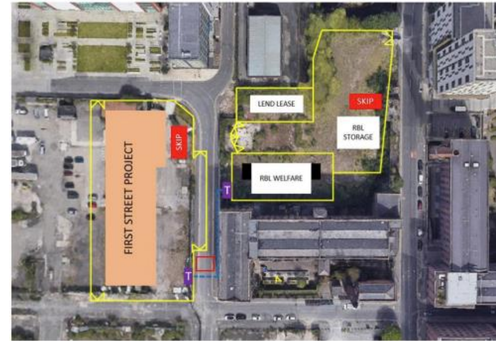
Figure 5.7 Skip locations for construction wastes
