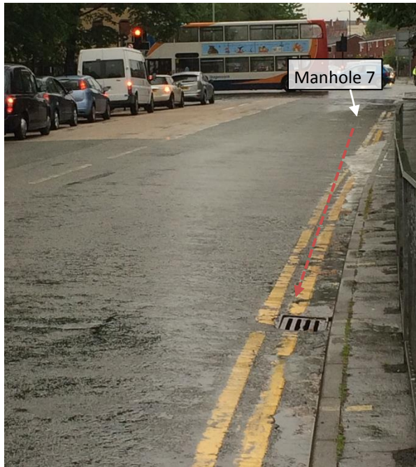
Image 3 - main overland flow paths for Manhole 7 (viewed East towards Upper Brook Street)
