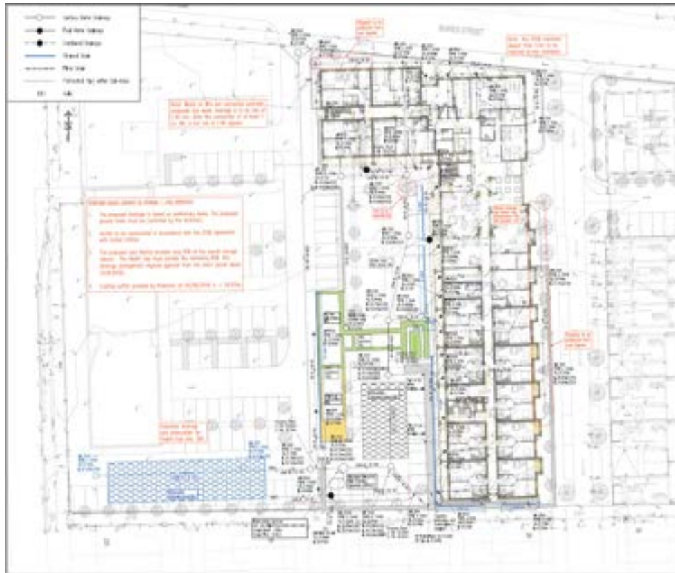
Figure 3.1 Care Facility Drainage Layout
