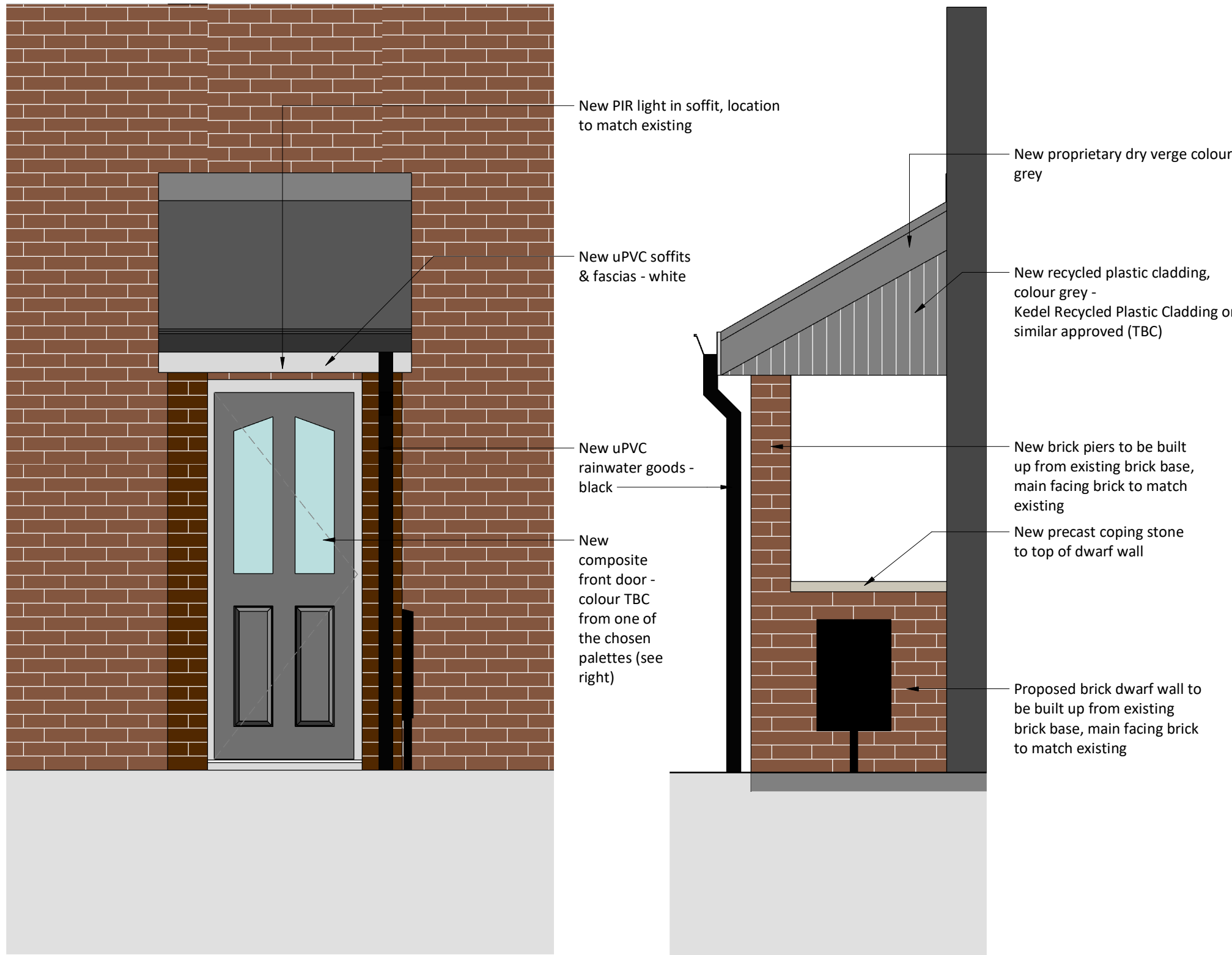
Front Elevation 1:25 TYPE 1 Flats 3, 6, 11, 14
