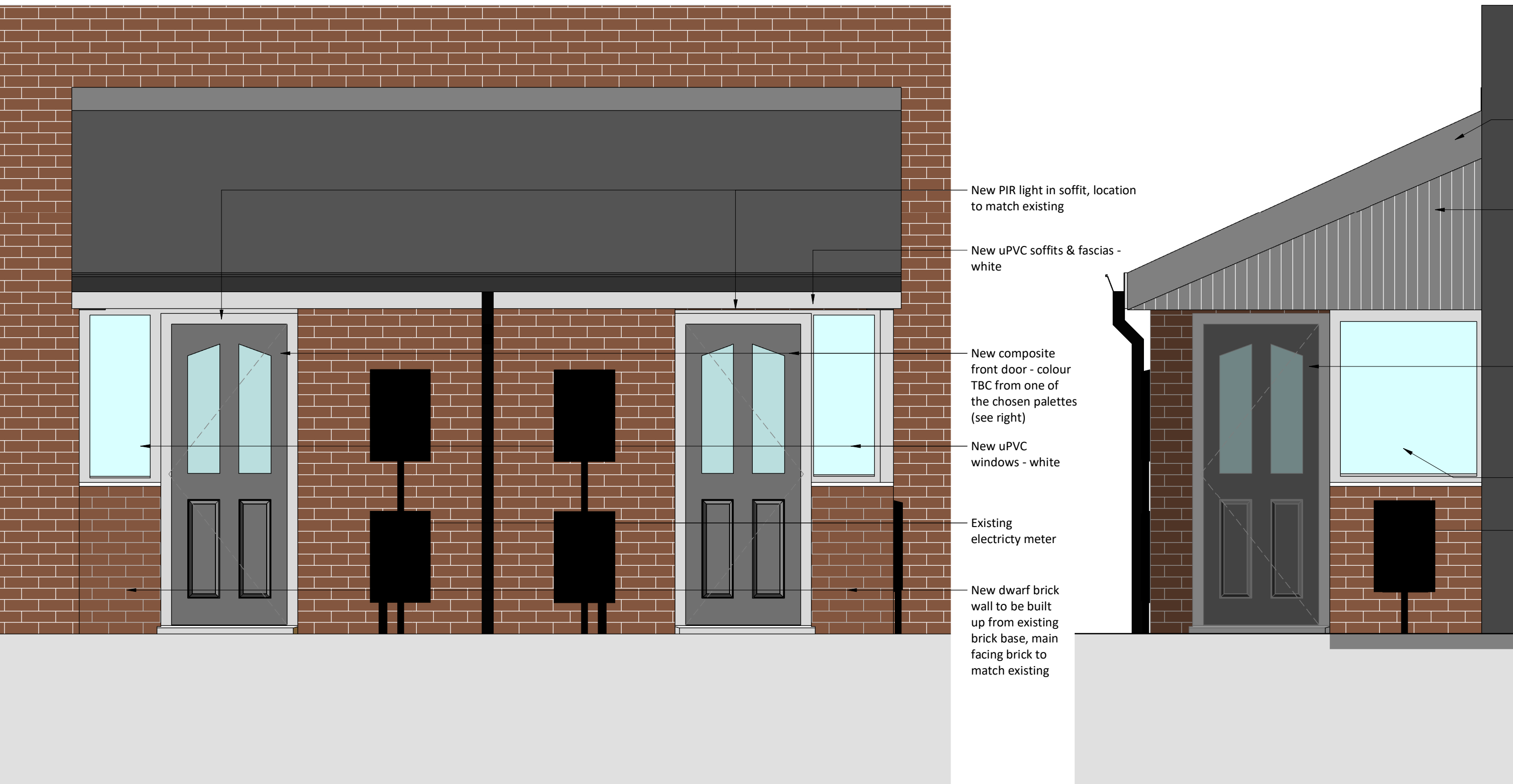
Front Elevation 1:25 TYPE 4 Flats 7, 8, 9 & 10
