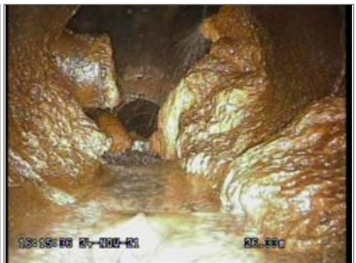
Attached deposits, encrustation from 1 to 6 o'clock 20% cross-sectional area loss
