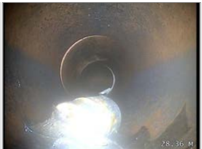
Other settled deposits 10% cross-sectional area loss - Remark: DEBRIS
