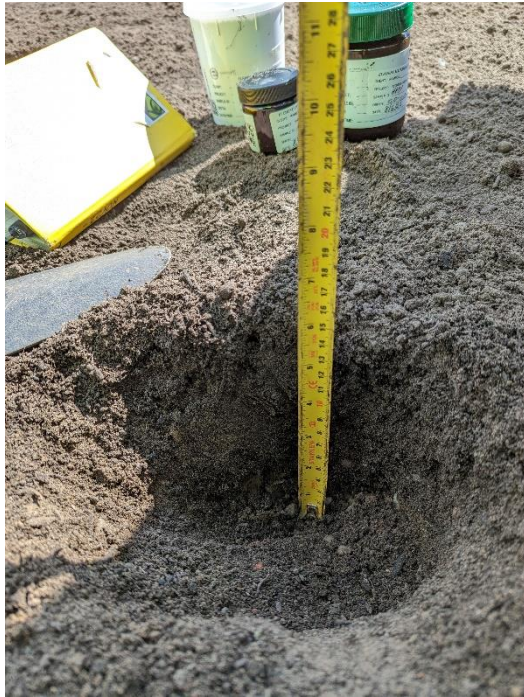
HP01 topsoil extending to 0.15 m (left) and HP02 topsoil extending to 0.12 m (right)
