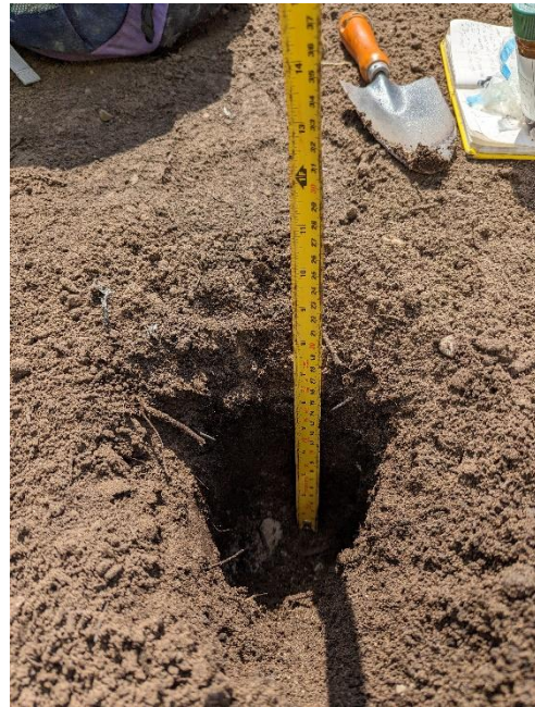
HP05 topsoil extending to 0.22 m (left) and HP06 topsoil extending to 0.20 m (right)
