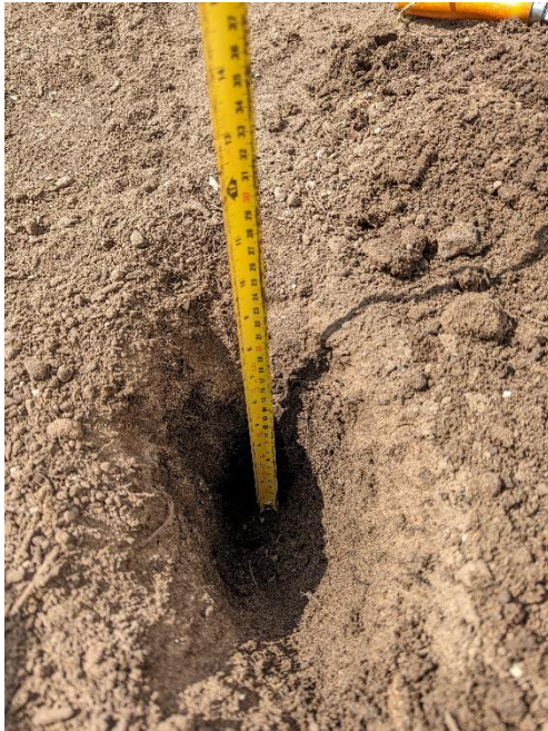
HP05 topsoil extending to 0.22 m (left) and HP06 topsoil extending to 0.20 m (right)
