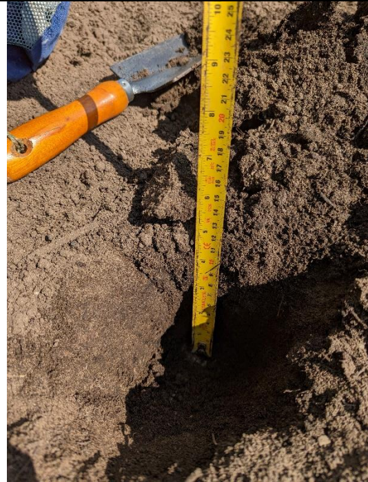
HP01 topsoil extending to 0.15 m (left) and HP02 topsoil extending to 0.12 m (right)
