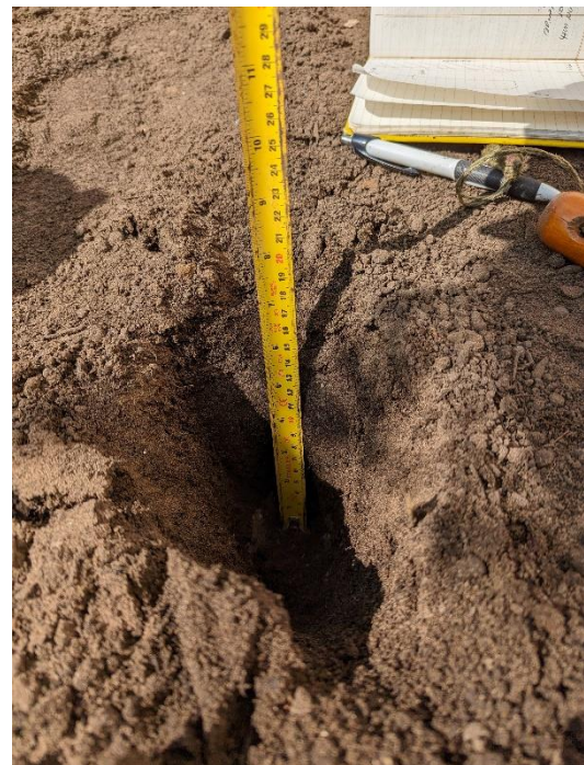
HP01 topsoil extending to 0.15 m (left) and HP02 topsoil extending to 0.12 m (right)
