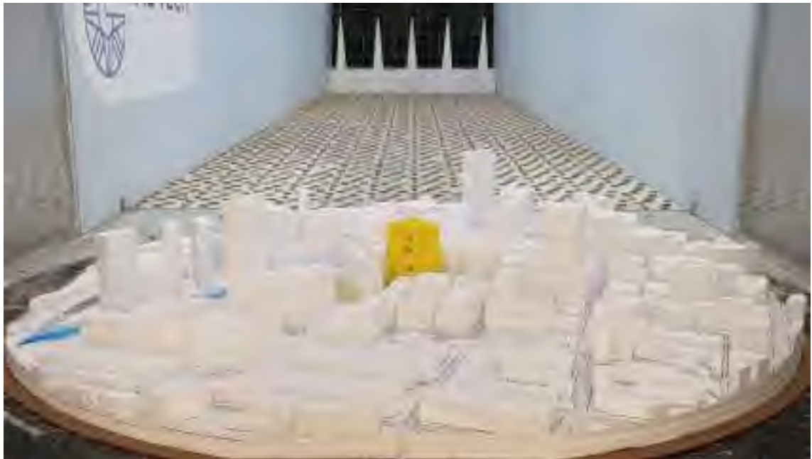
Figure 1c: Photograph of the Wind Tunnel Model: The Proposed Development with Existing Surrounds (view from the south)
