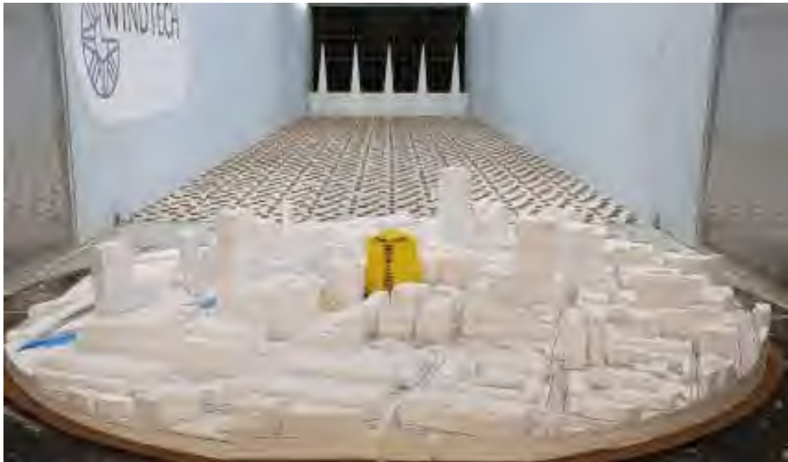
Figure 1g: Photograph of the Wind Tunnel Model: The Proposed Development with Existing Surrounds and Mitigation (view from the south)
