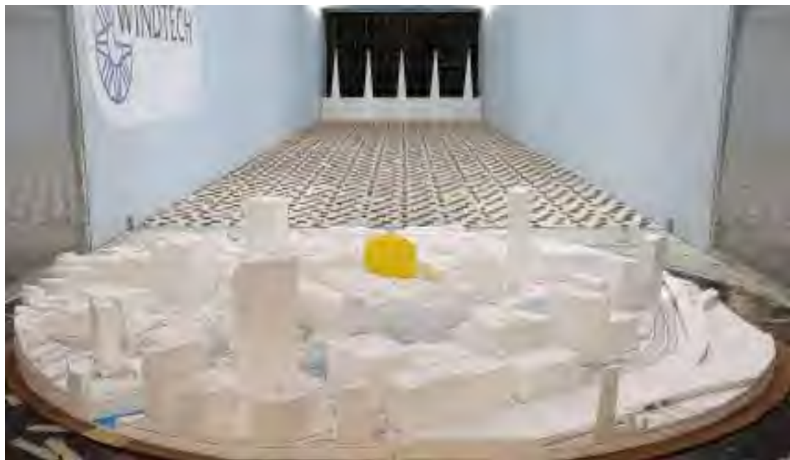
Figure 1h: Photograph of the Wind Tunnel Model: The Proposed Development with Existing Surrounds and Mitigation (view from the north)
