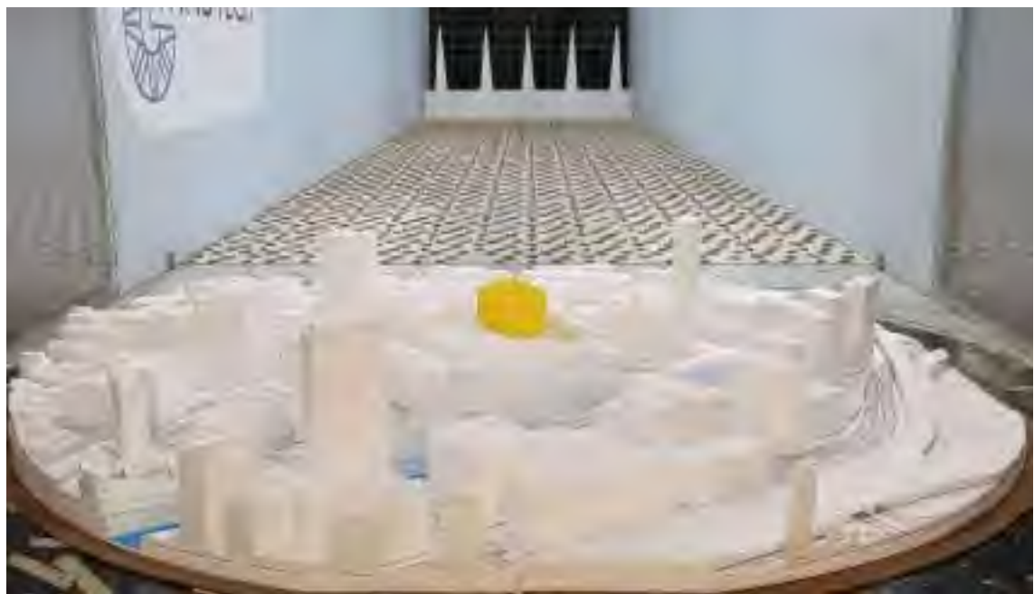
Figure 1d: Photograph of the Wind Tunnel Model: The Proposed Development with Existing Surrounds (view from the north)
