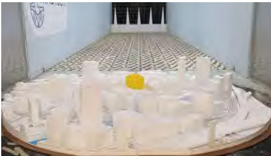
Figure 1f: Photograph of the Wind Tunnel Model – The Proposed Development with Future Surrounds (view from the north)
