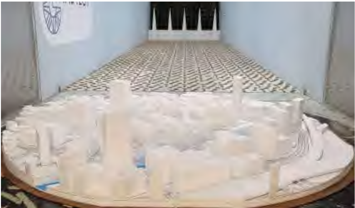
Figure 1b: Photograph of the Wind Tunnel Model: The Existing Site with Existing Surrounds (view from the north)
