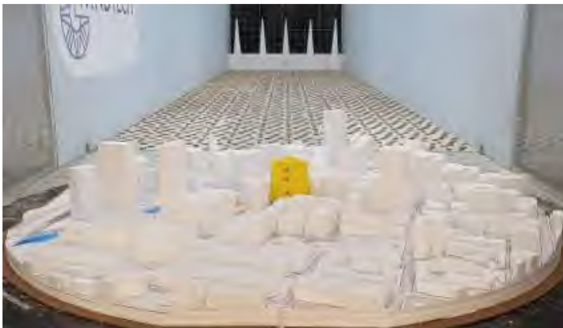
Figure 1e: Photograph of the Wind Tunnel Model: The Proposed Development with Future Surrounds (view from the south)
