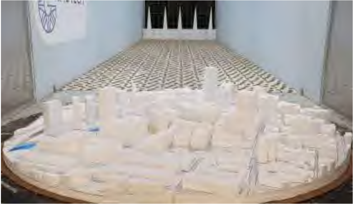
Figure 1a: Photograph of the Wind Tunnel Model: The Existing Site with Existing Surrounds (view from the south)
