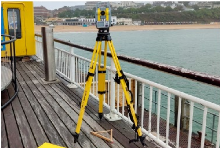
8: Field survey being carried out, total station
