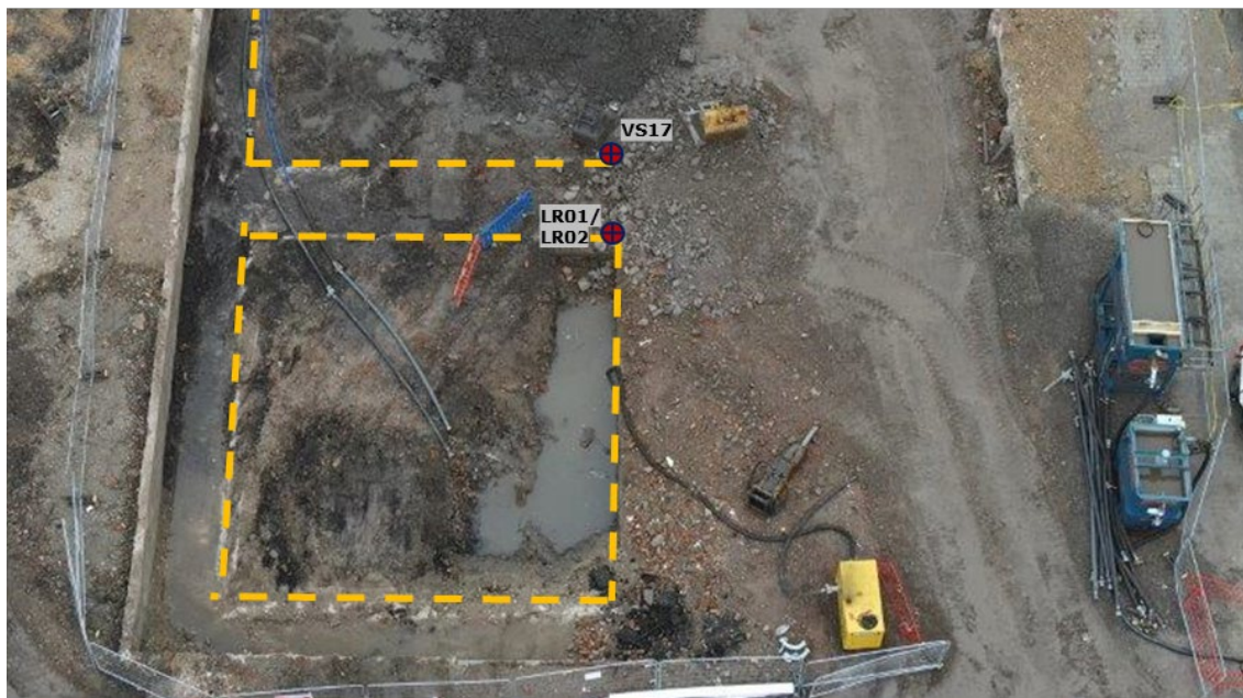
Figure 2: Approximate sampling locations in the Basement Area during the August sampling event. Aerial image taken facing the north-east. Dashed line depicts the concrete slab edges.
