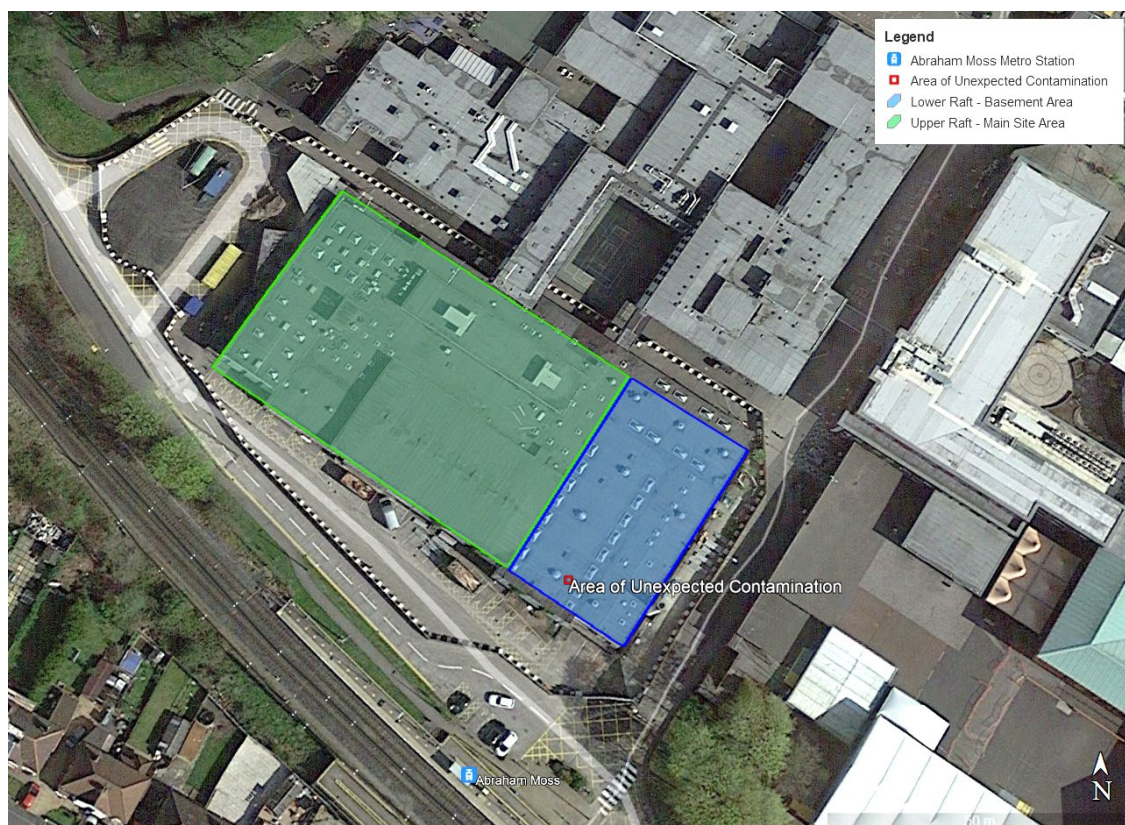
Figure 1: Indicative Site Layout Plan (shown prior to demolition)
