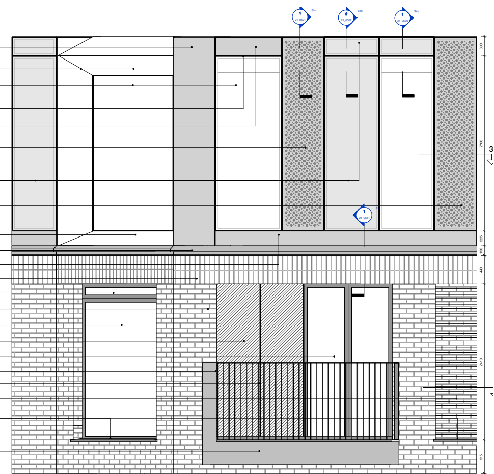
3 | Mock-Up Panel - Elevation 1 : 20
