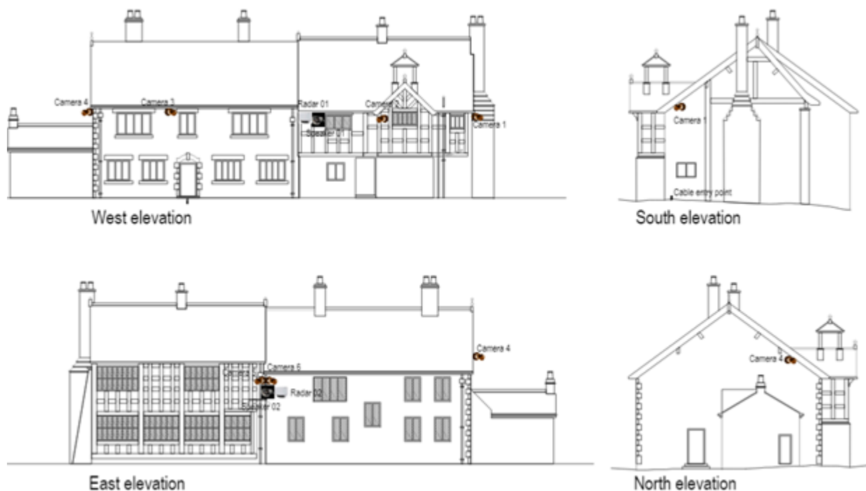
Fig. 3 – Elevations with proposed security features
