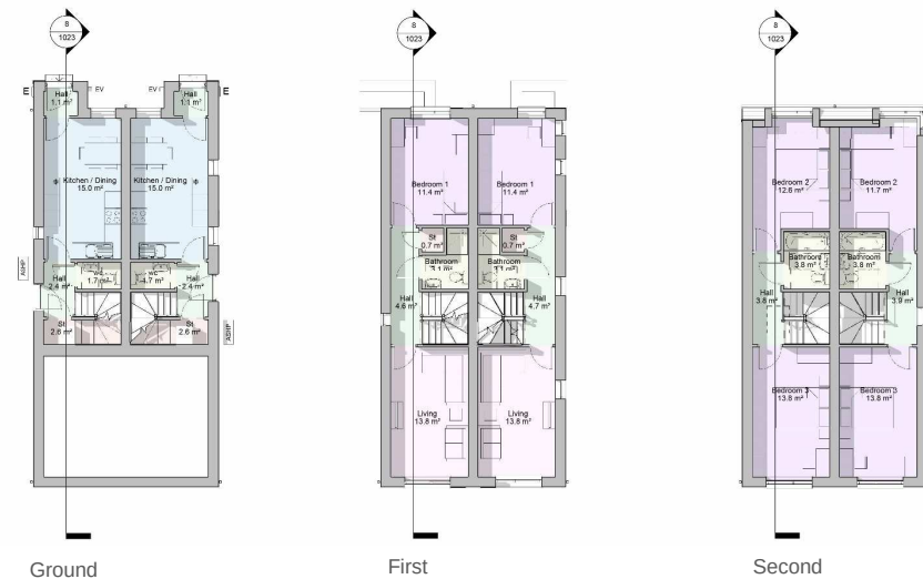
Fig.19: Houses- middle units- floor plans
