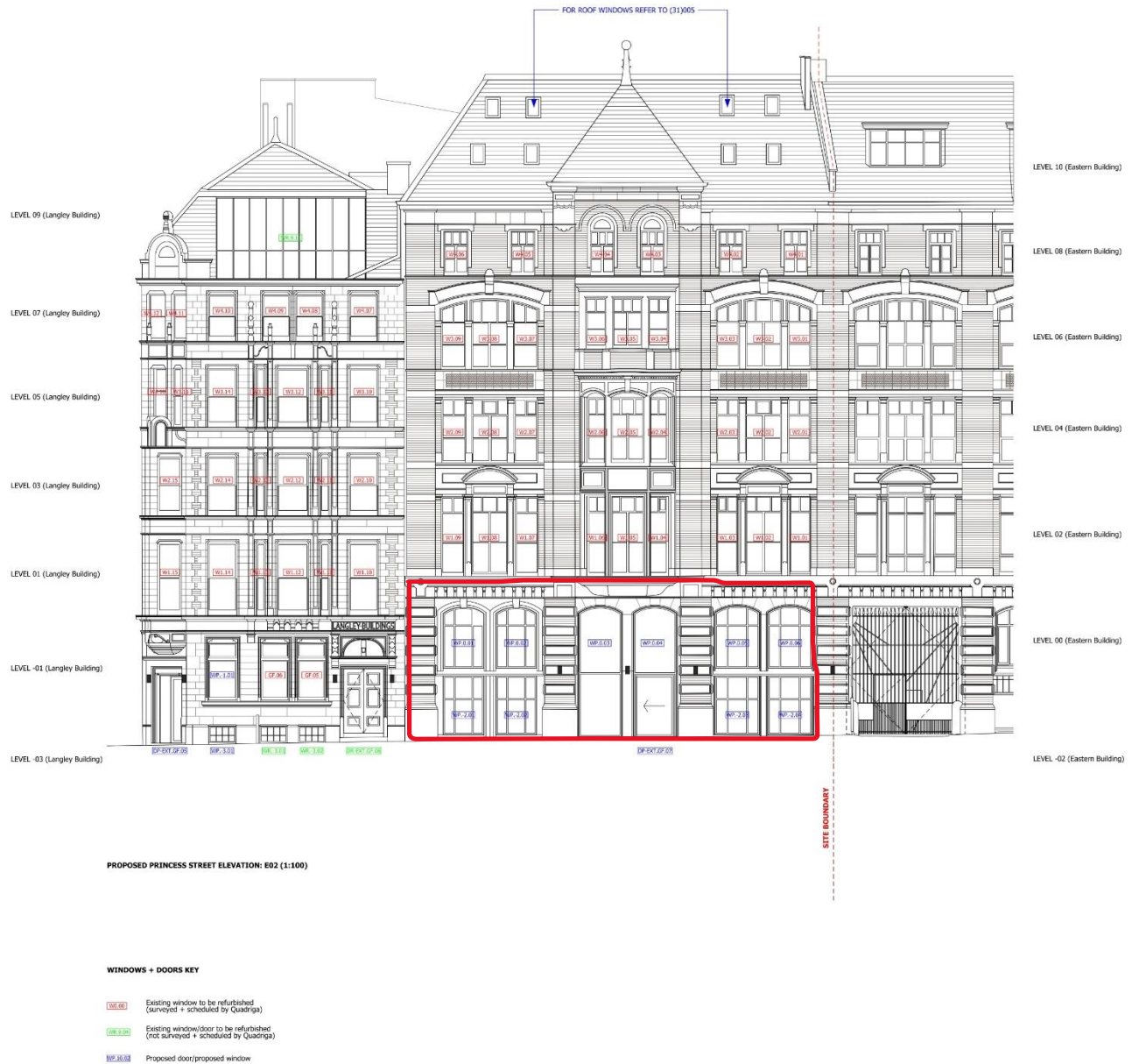
Figure 67: Location of Windows replaced on the Princess Street Elevation (Credit Bridge Architects 2021)
