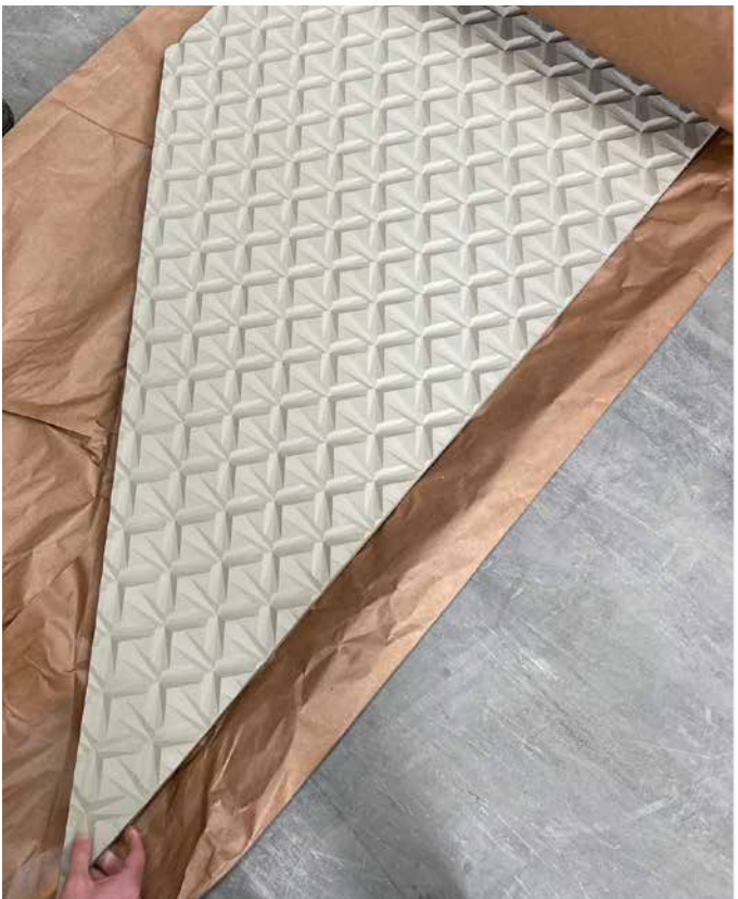
Precast pattern mould
