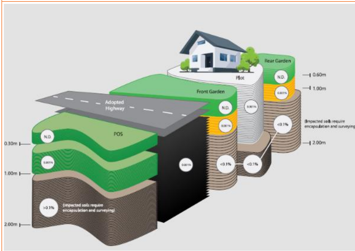
FIGURE 4.1 ASBESTOS RISK MITIGATION CONCEPTUAL SITE MODEL
