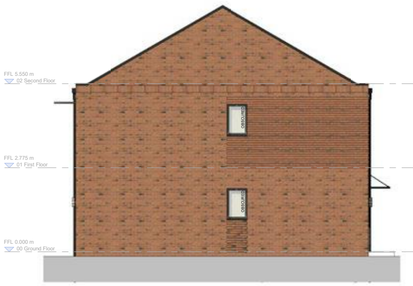
Gable Elevation - End Terrace - Plots 6, 17 & 22
