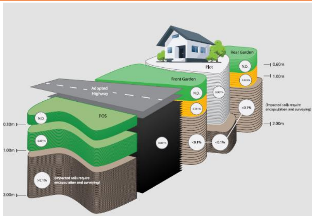
FIGURE 4.1 ASBESTOS RISK MITIGATION CONCEPTUAL SITE MODEL
