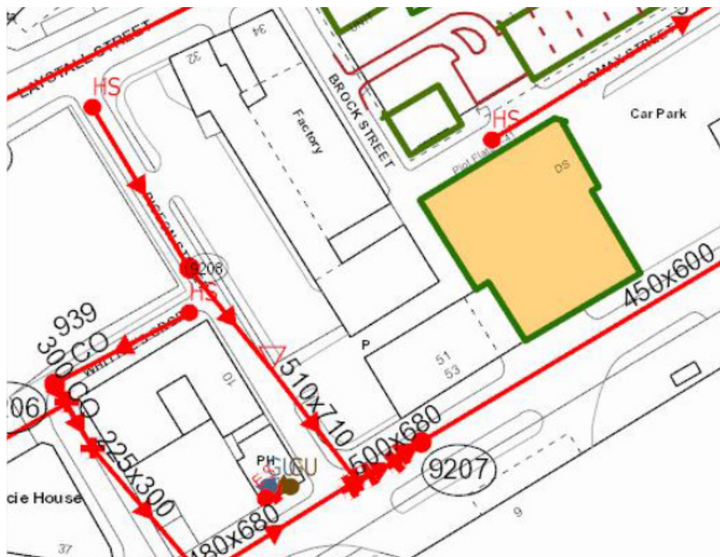
Figure 2 – Public Sewer Network. Source: United Utilities.
