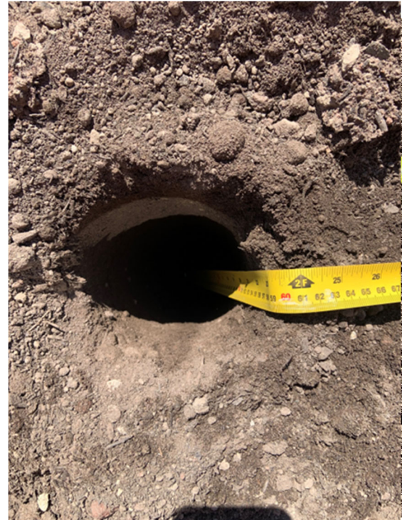
Photograph 2: Plot 369 Validation Pit Depth
