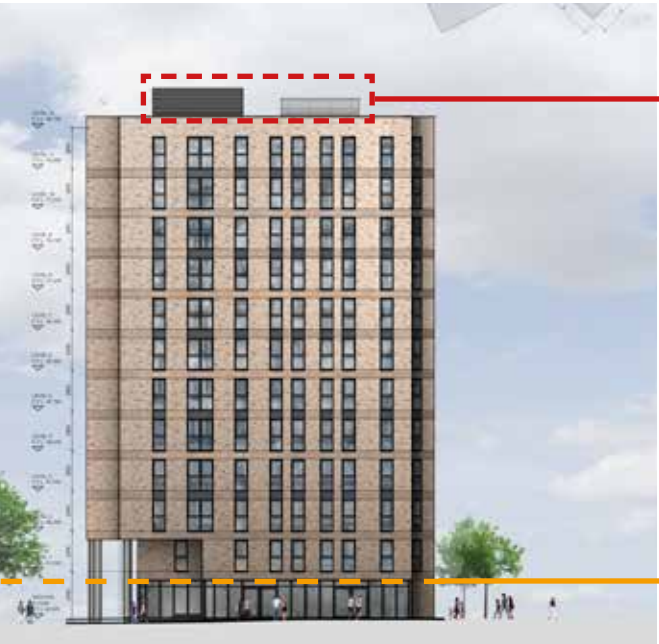
Elevation B Planning Refinements REMOVAL OF LIFT AND STAIRCASE GROUND FLOOR HEIGHT REDUCED BY 450MM
