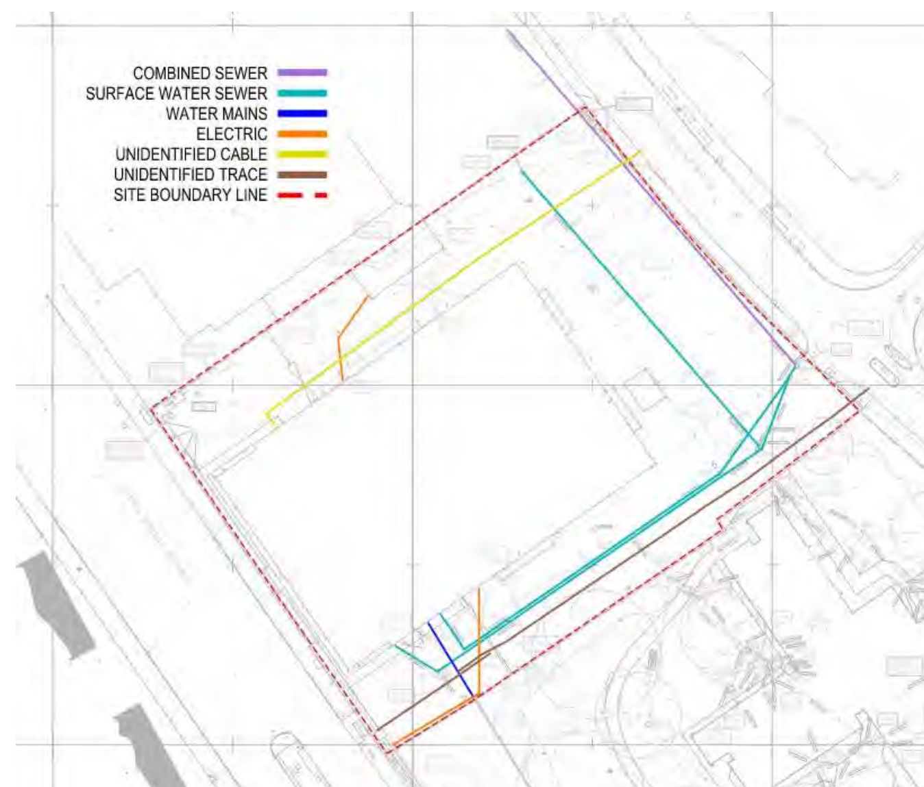
Figure 7 - CCTV survey overlay plan
