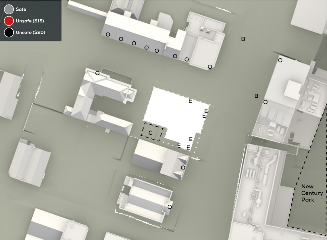
Figure 12.7 Strong Winds at Ground Level for Scenario 2 (Proposed Development with Existing Surrounds)
