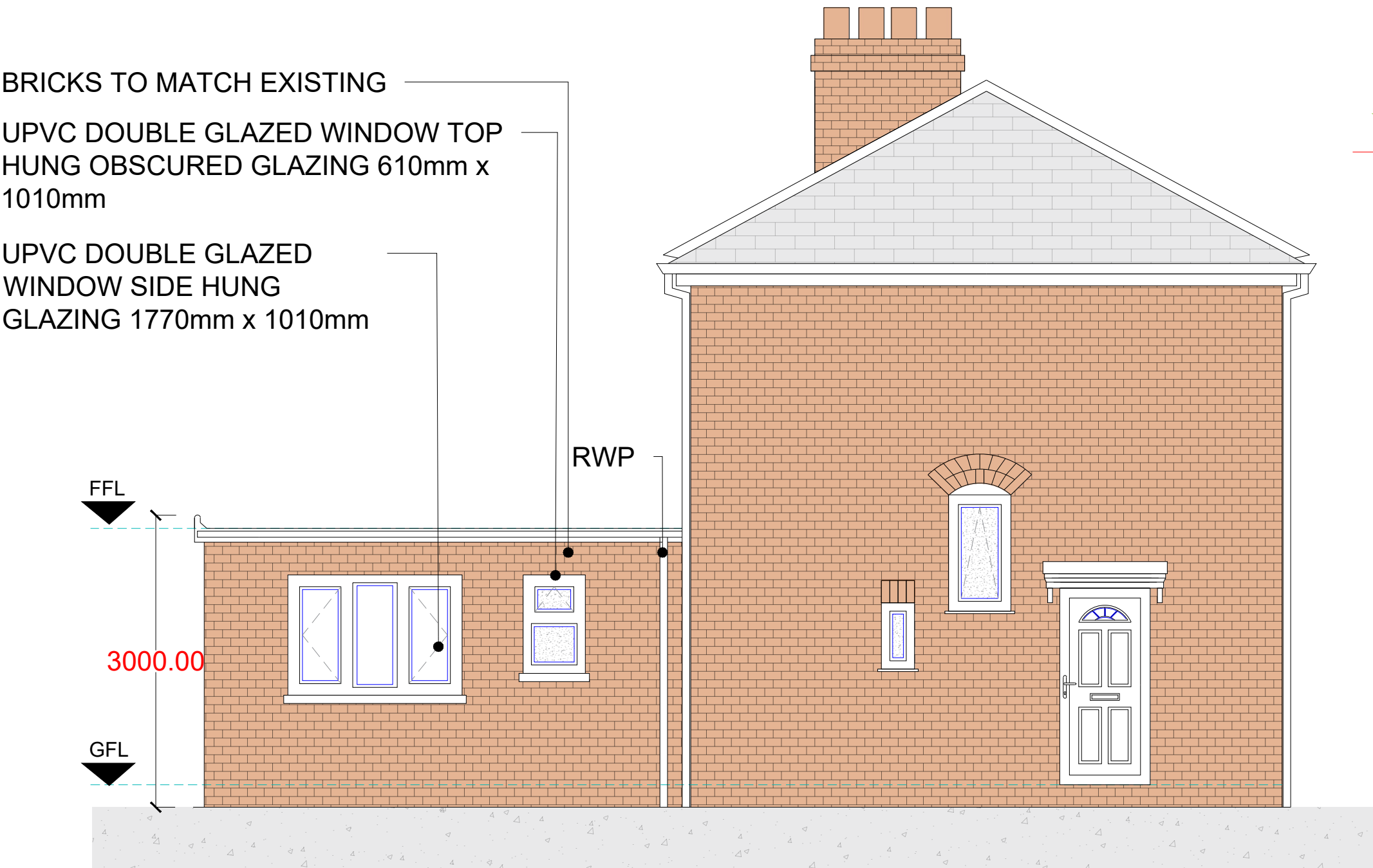
Proposed Front Elevation Scale 1:50
