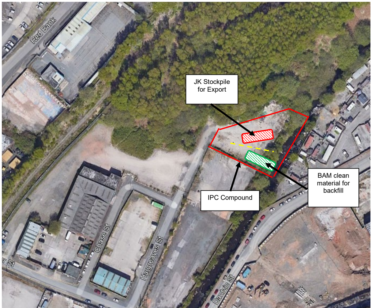
Figure 2: Showing the IPC compound and potential stockpile locations
