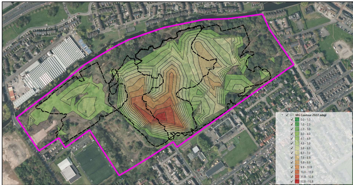
Figure 1: Extract of Made Ground Thickness Contour showing areas where Made Ground exceeds c. 3m in thickness. This equates to c. 55% of the site area. Black dashed lines show the recorded extent of the former clay pit excavations.
