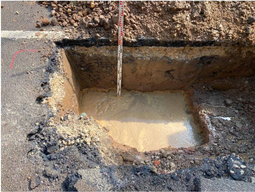
Plate 5 – TP02 undergoing BRE infiltration testing (SA01).
