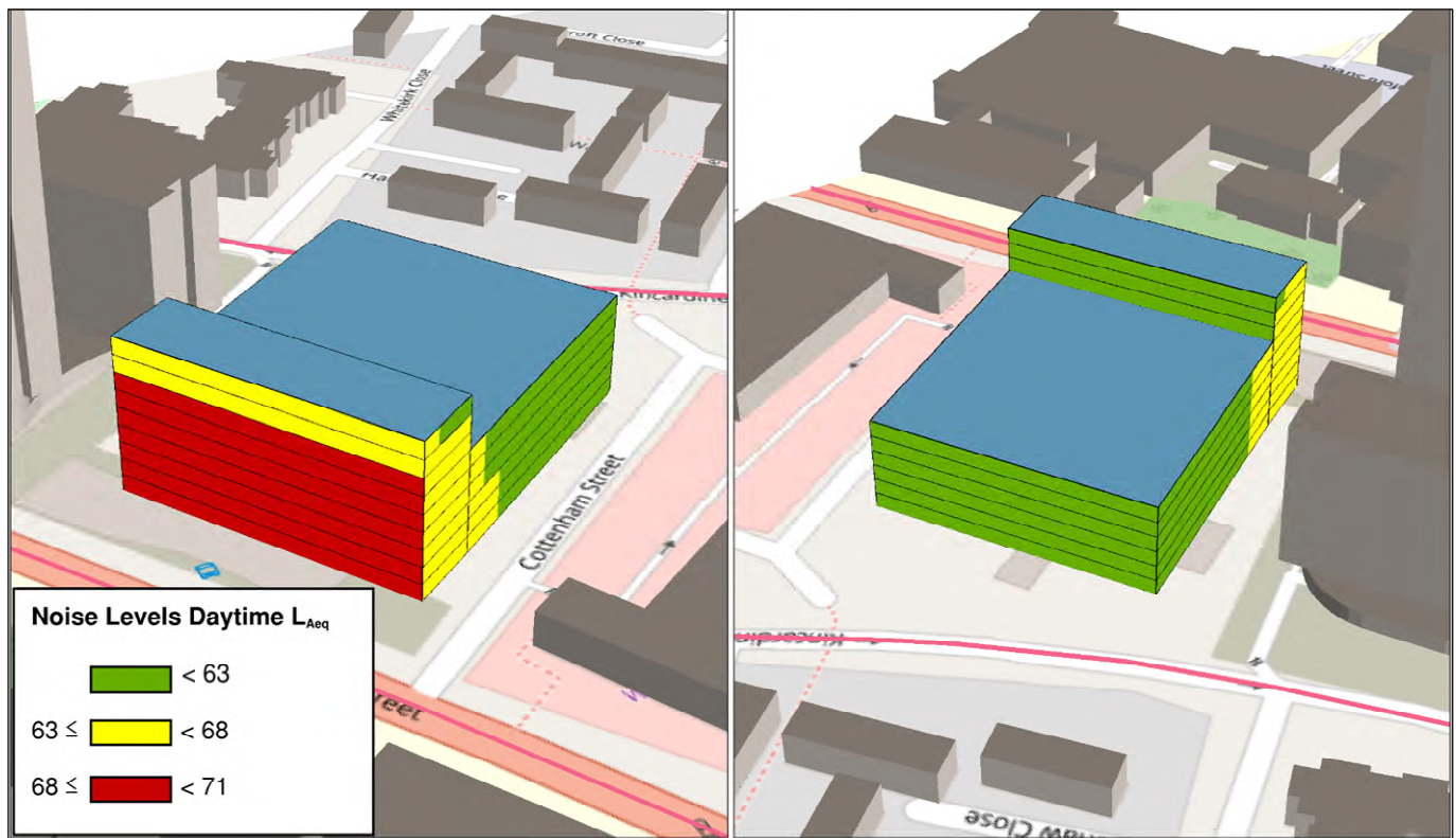
Figure 5—5: Predicted free-field noise levels from road traffic on façades of Sci-Tech Building
