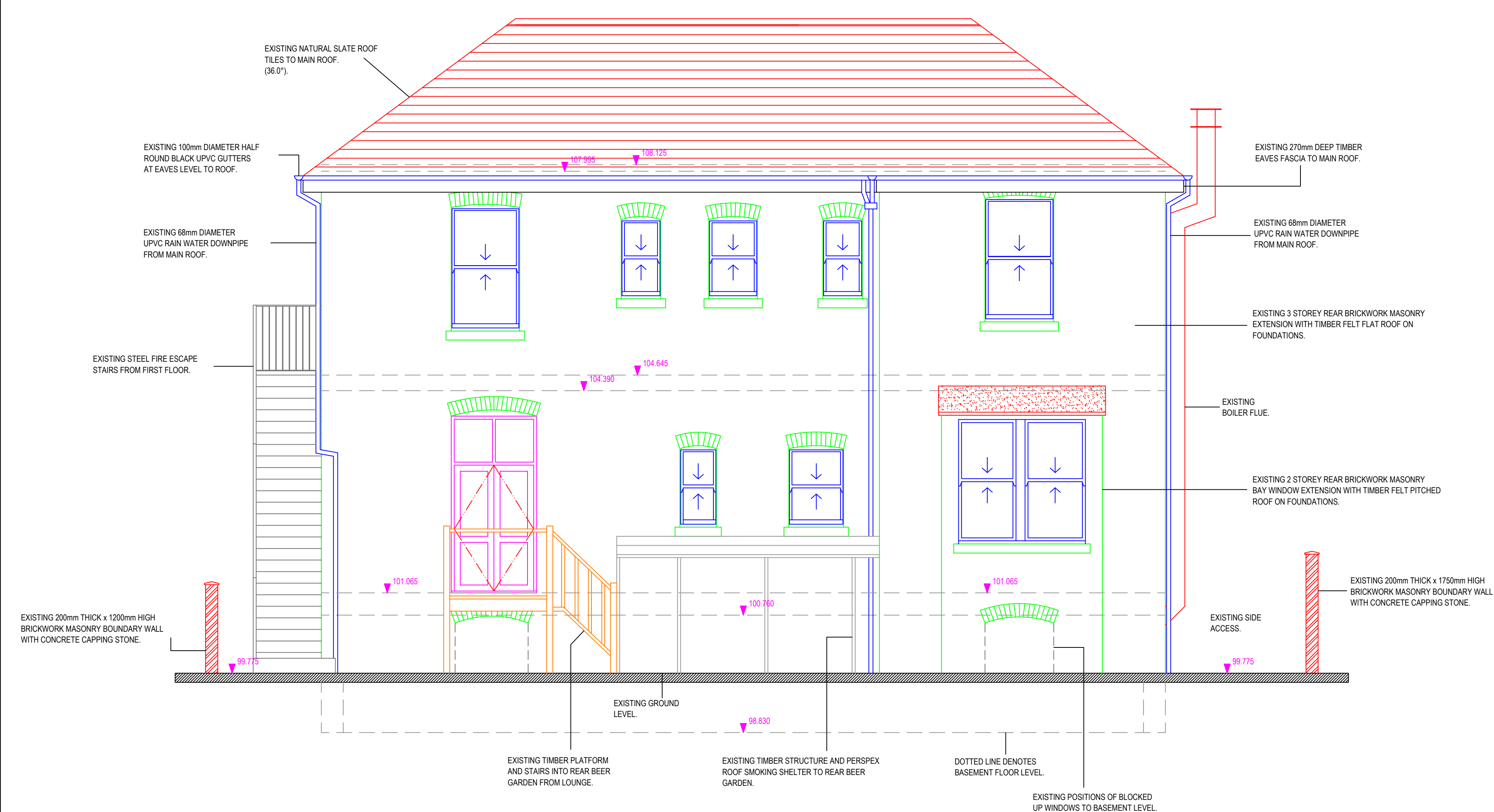
EXISTING SOUTH EAST ELEVATION
