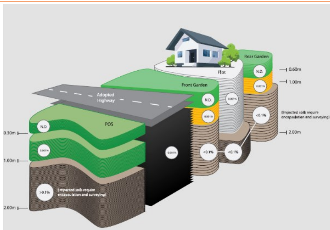
FIGURE 4.1 ASBESTOS RISK MITIGATION CONCEPTUAL SITE MODEL
