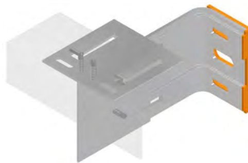
Fixing Arrangement on A Fixed Adaptor
