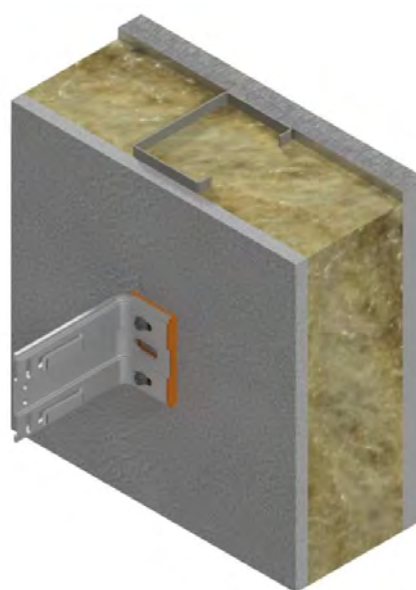
Based Fixings for A Single Bracket to SFS
