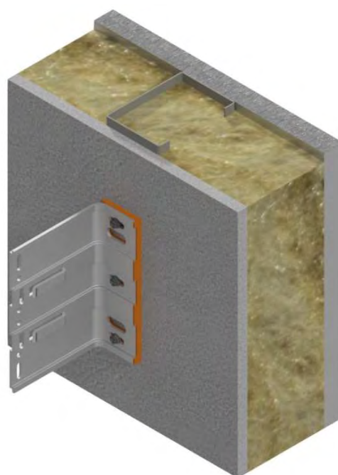
Base Fixings for A Double Bracket on SFS
