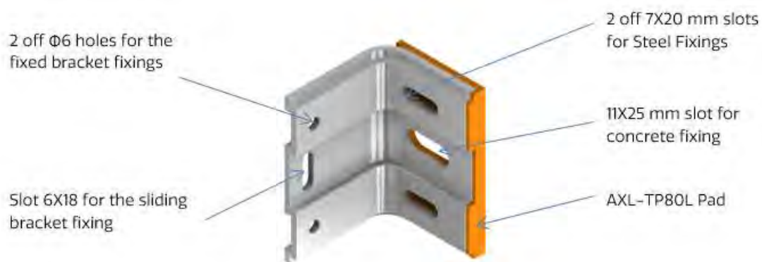
Single Bracket with length \leq 60 mm
