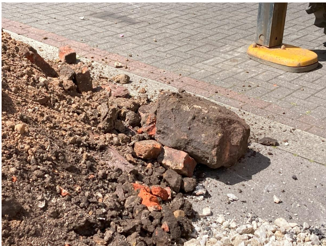
Plate 9 – Coarse gravel, cobbles and boulders within TP04 arisings.
