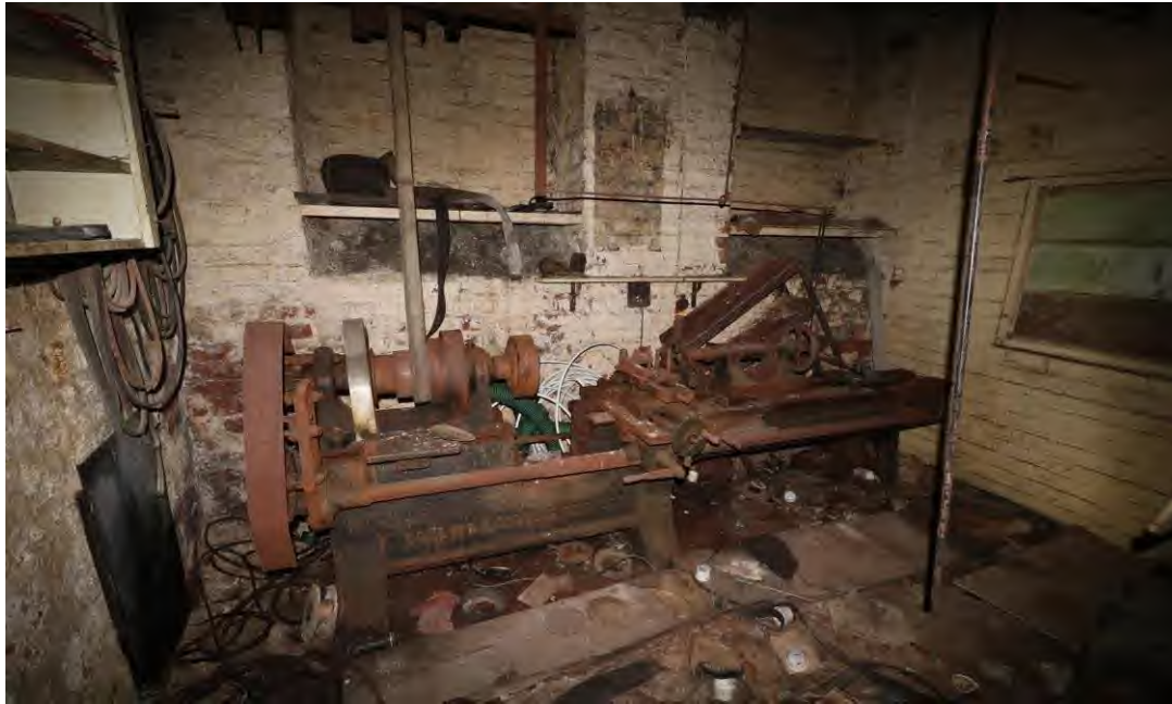
Figure 89: An original 1900s steam driven lathe in the basement area.
