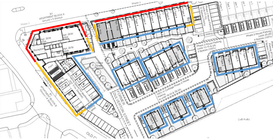
Façade acoustic specification zones (all levels)
